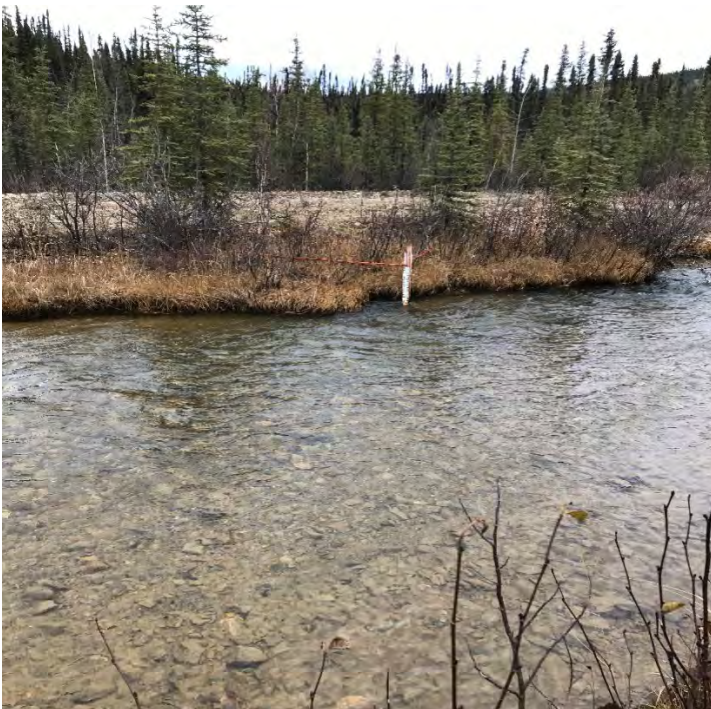
Photo 8 Staff Gauge for Site W4 on Haggart Creek below Dublin Gulch Confluence
