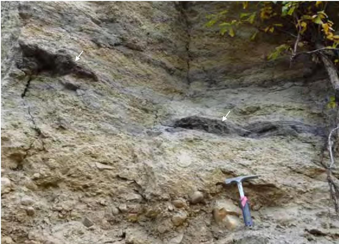
Note: Cobble layer overlain by bedded sand and silt with organic lenses (arrows).
