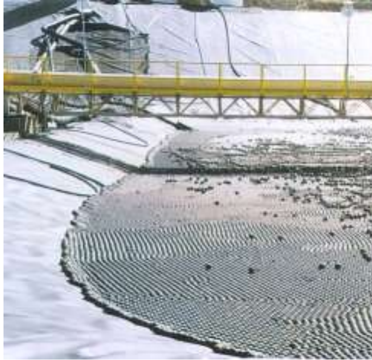
Photo 6.9-1: Bird Balls floating on the surface of a heap leach pregnant solution pond to prevent waterfowl fatalities
