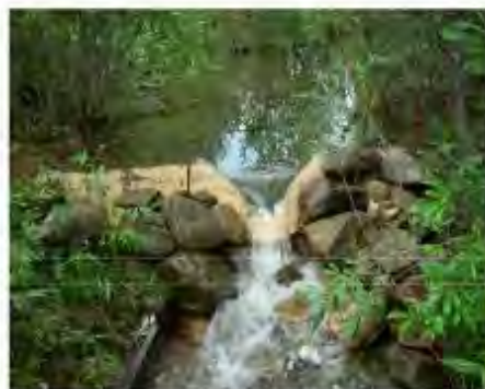
Weir on Eagle Pup used to measure flow volume, 2009
