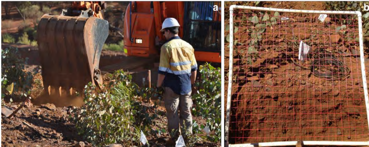
Figure 2.1-1: Creation of pit into a cover system with established vegetation to quantify root depths, distribution, and material textures
