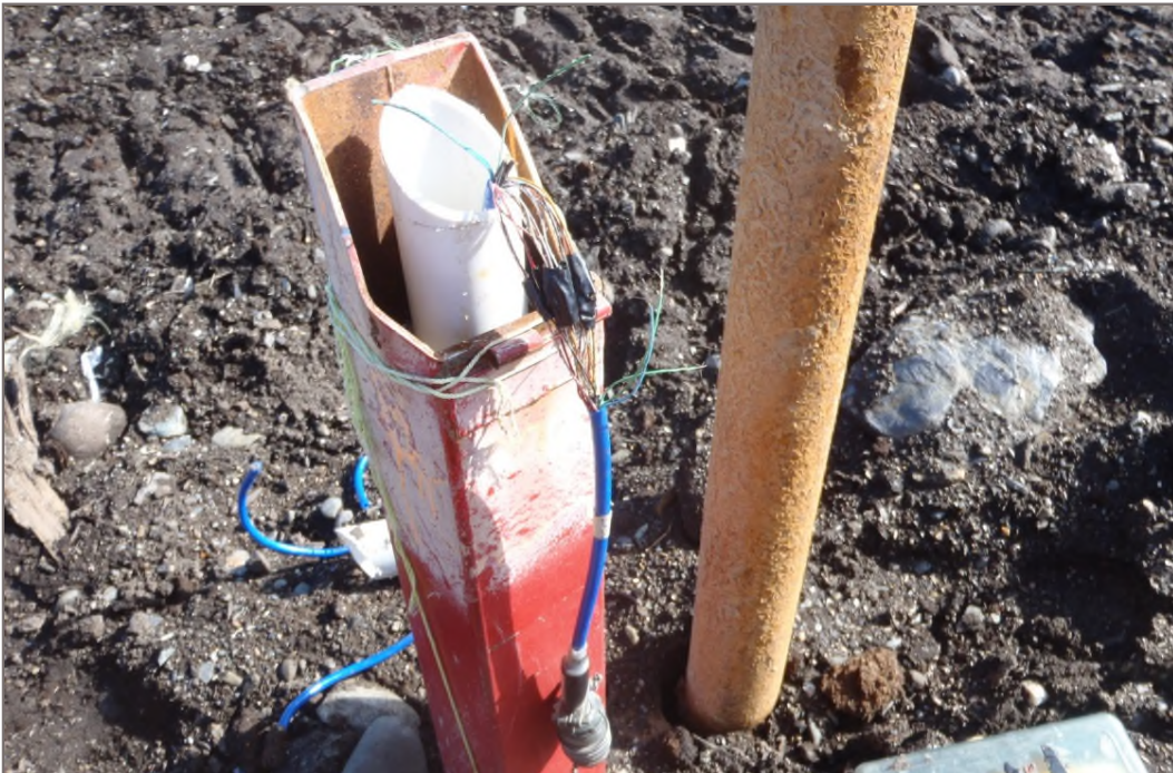
Photo 26: Dry Stacked Tailings Facility Attempted repair of the ground temperature cable in BH40 Facing north – August 13, 2014
