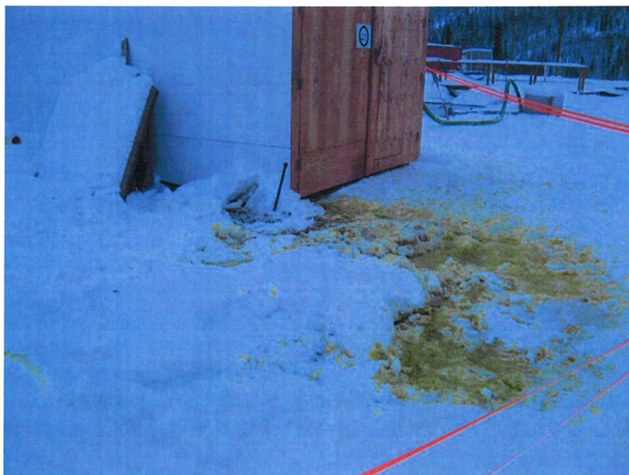
BK625 Ferric Chloride Mixed with Snow Outside of Reagent Shed
