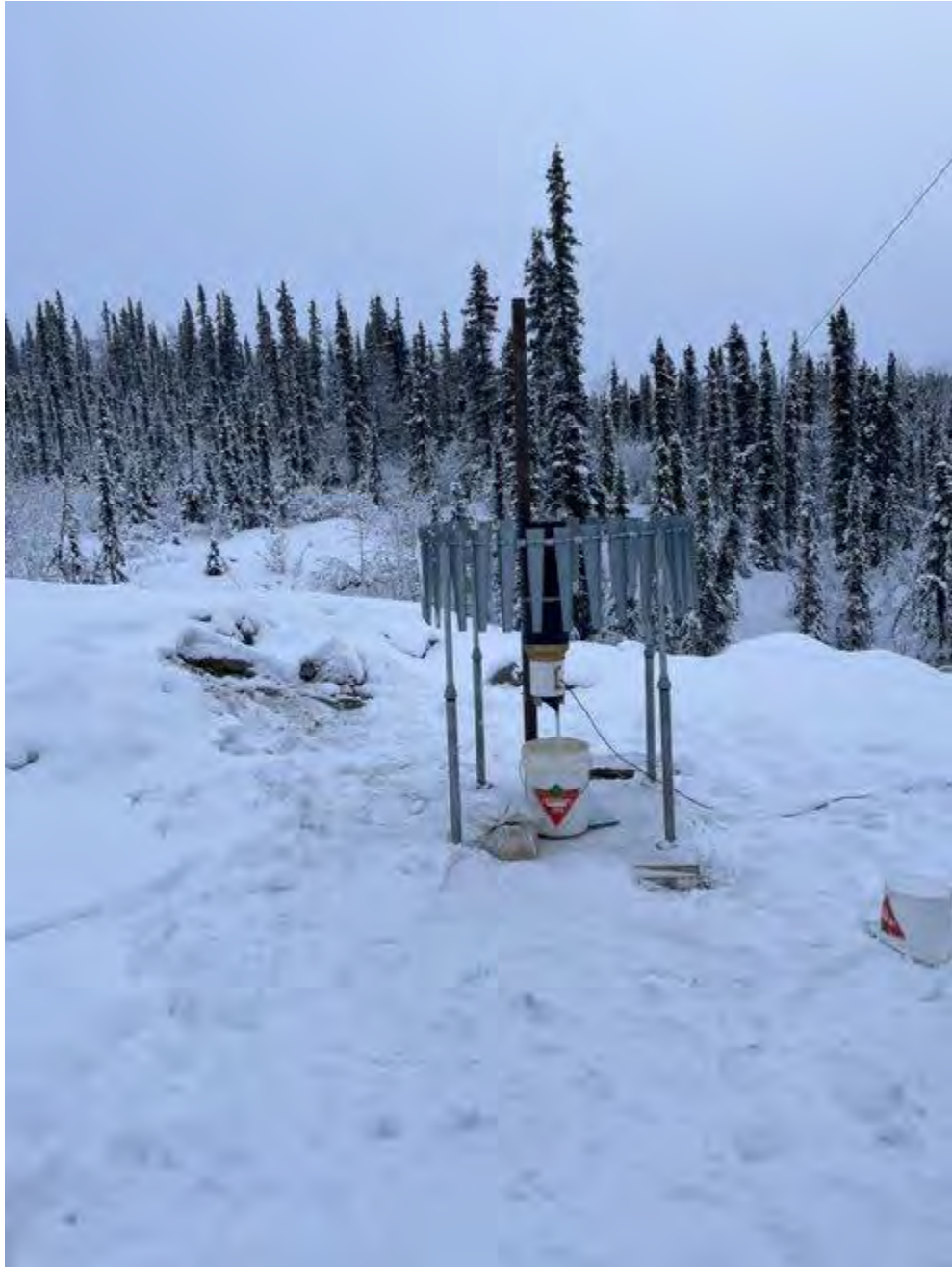
Figure 3: District Mill Tipping Bucket and Alter Wind Screen (added November 2022)
