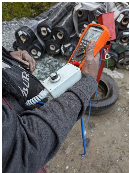
Figure 3 Mine Technician collecting real-time readings from the Ground Temperature Probes.
