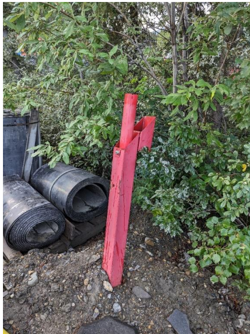
Figure 4 Slope inclinometer station, BH36.
