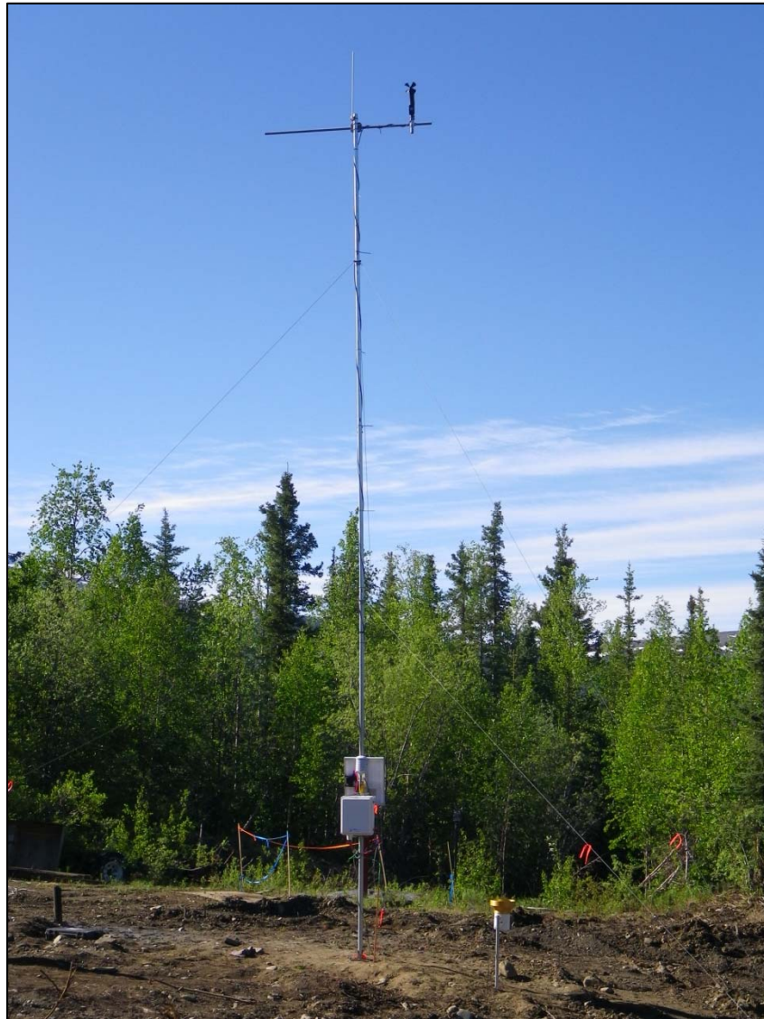
District Mill Campbell Scientific Meteorological Station
