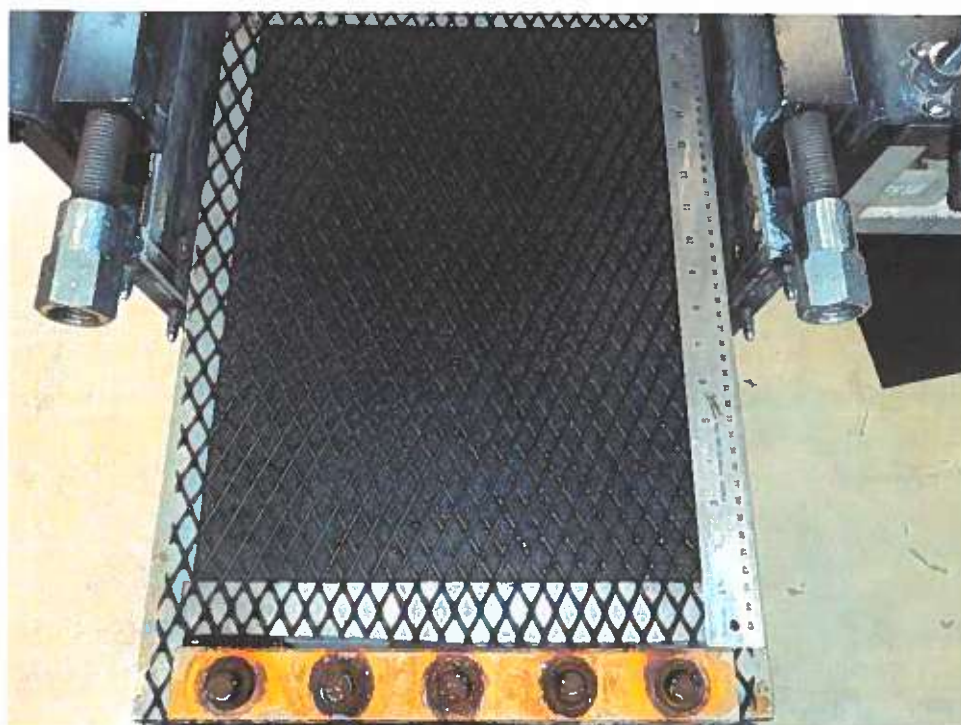
Geonet after the test – Test at 400kPa
