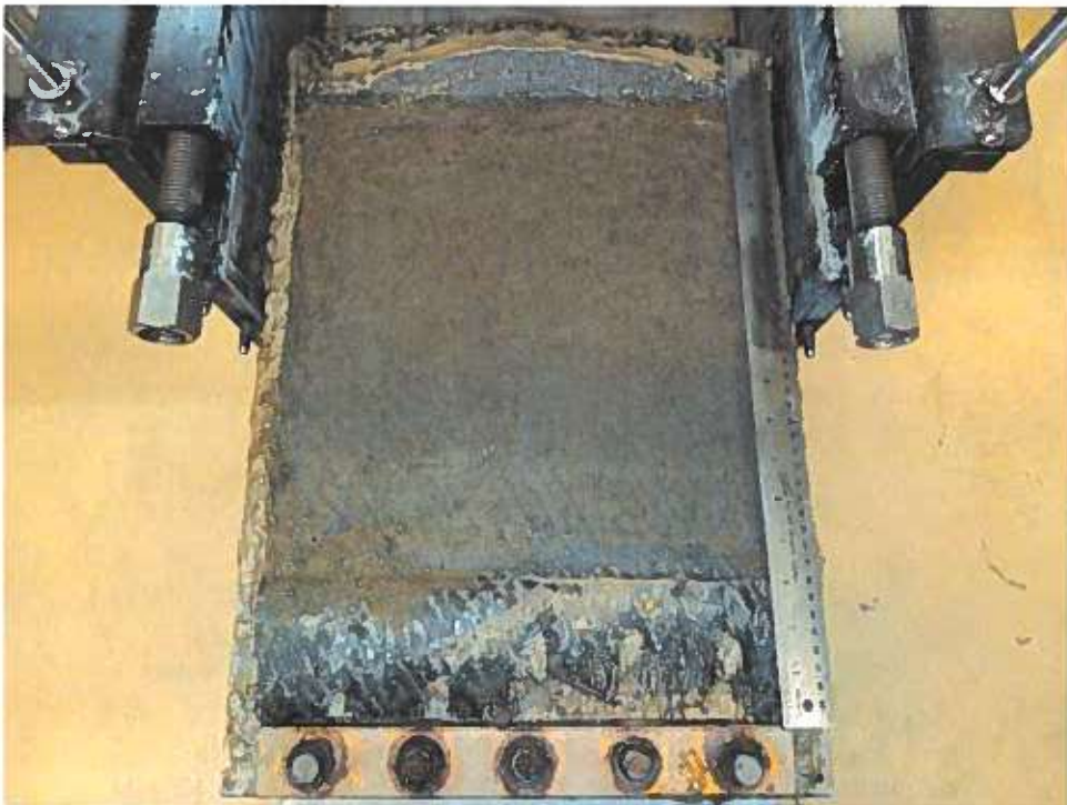
GCL Bentomat ST#10 (woven side) after the test – Test at 200kPa
