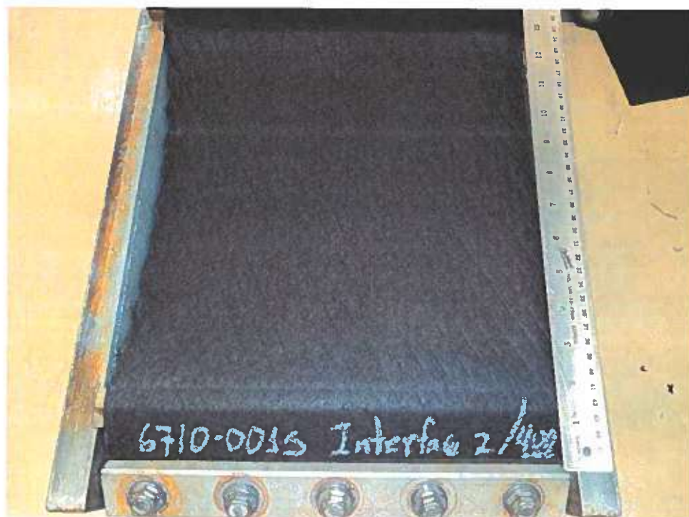
Non-woven Geotextile after the test – Test at 400kPa
