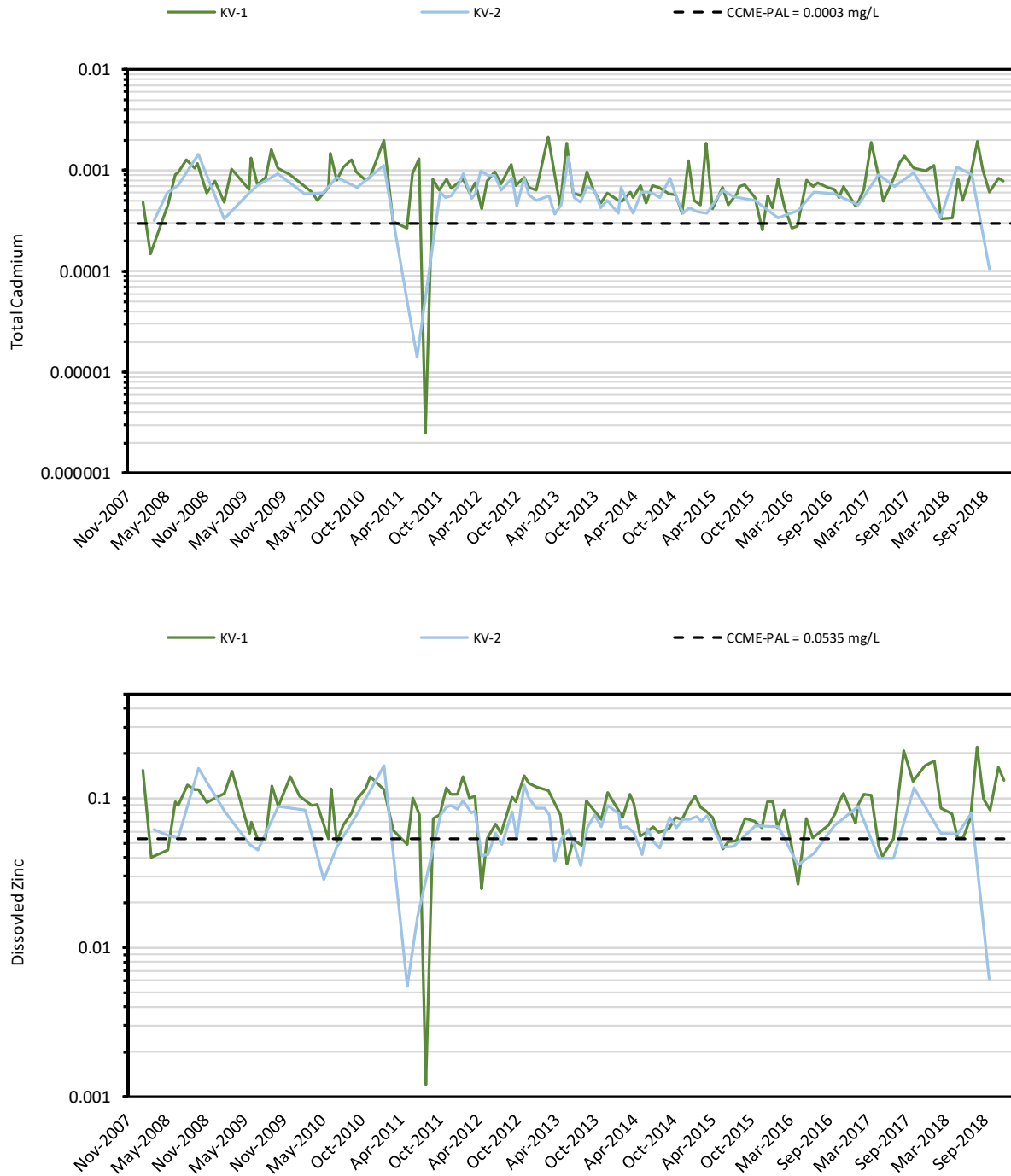
Figure 4-7: Total Cadmium and Dissolved Zinc Concentrations (in mg/L) at Stations KV-1 and KV-2 in the South McQuesten River
