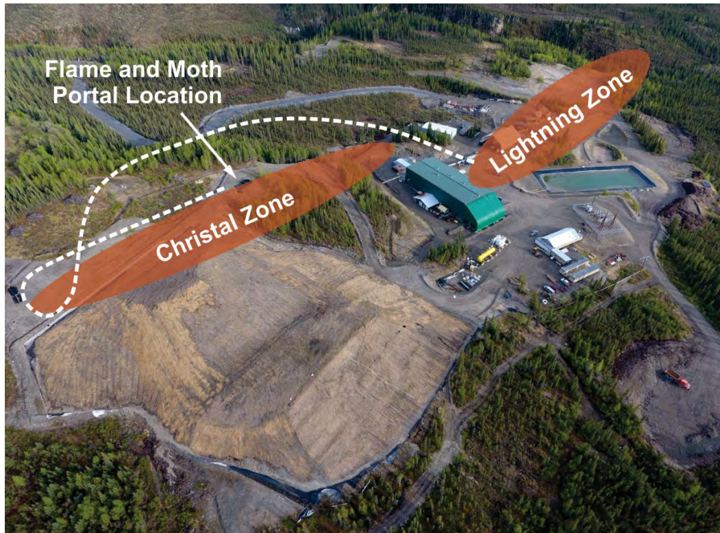
Figure 7-7 Flame & Moth Plan View Showing Ore Zones To Be Mined
