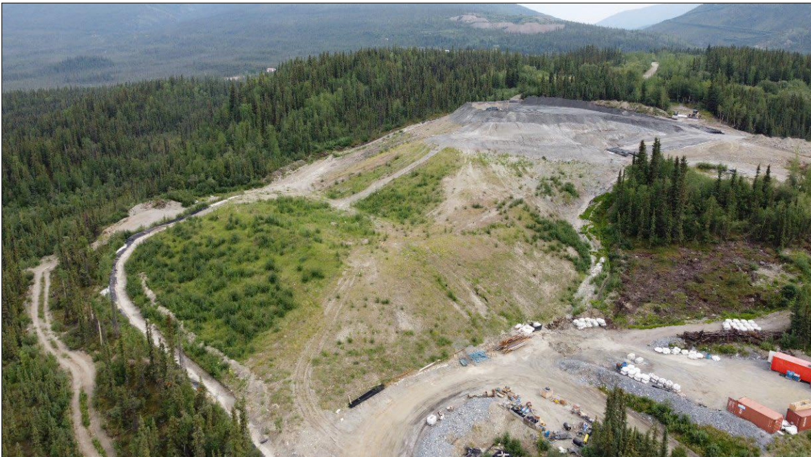
Photo 6-4: DSTF Progressive Reclamation, August 2023
