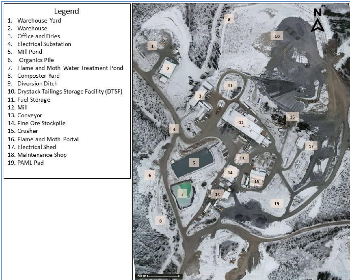
Figure 8-12: Aerial View of Mill Site Infrastructure and Layout
