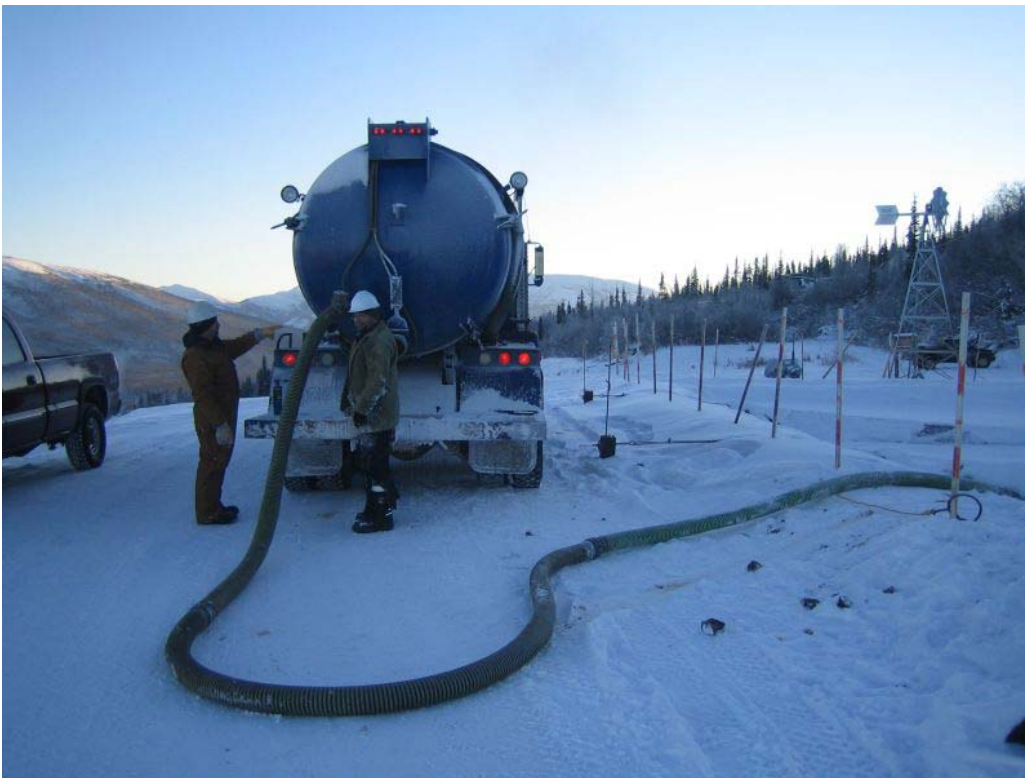
FIGURE 4 - VACUUM TRUCK USED TO DESLUDGING PONDS
