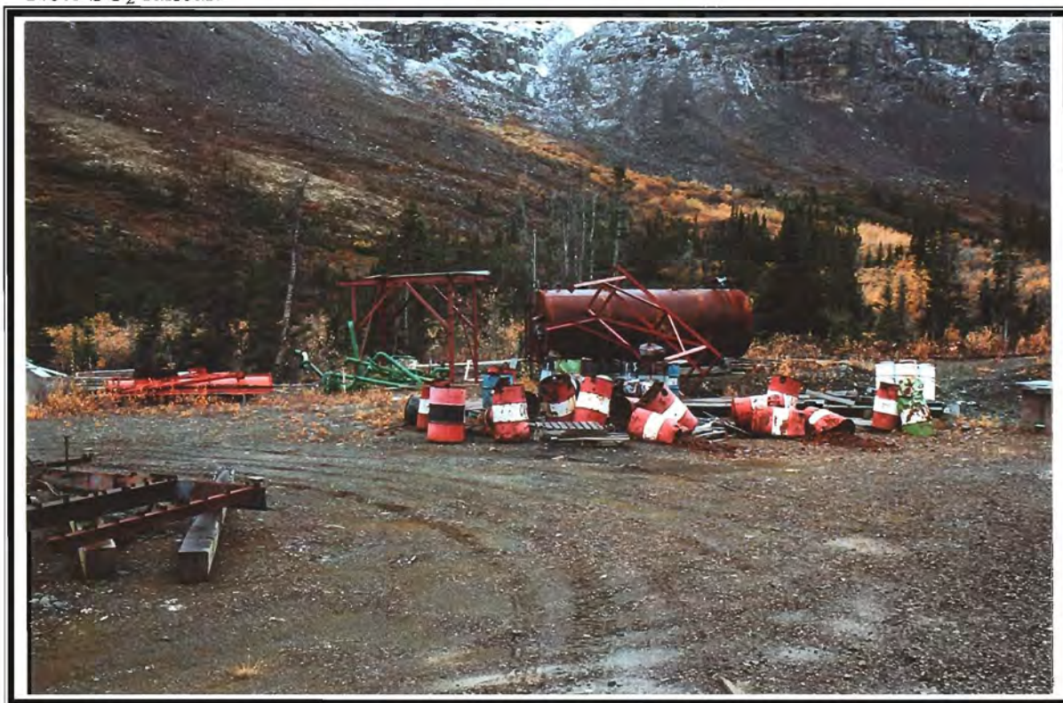
Photo 20: Portion of mill boneyard. Note drums of used mill balls in foreground. Tank in background is temporary storage.
