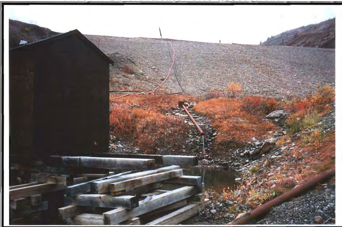
Photo 38: Tailings pond seepage sample (KR-04) taken from pipe-discharge from toe of North Dam.
