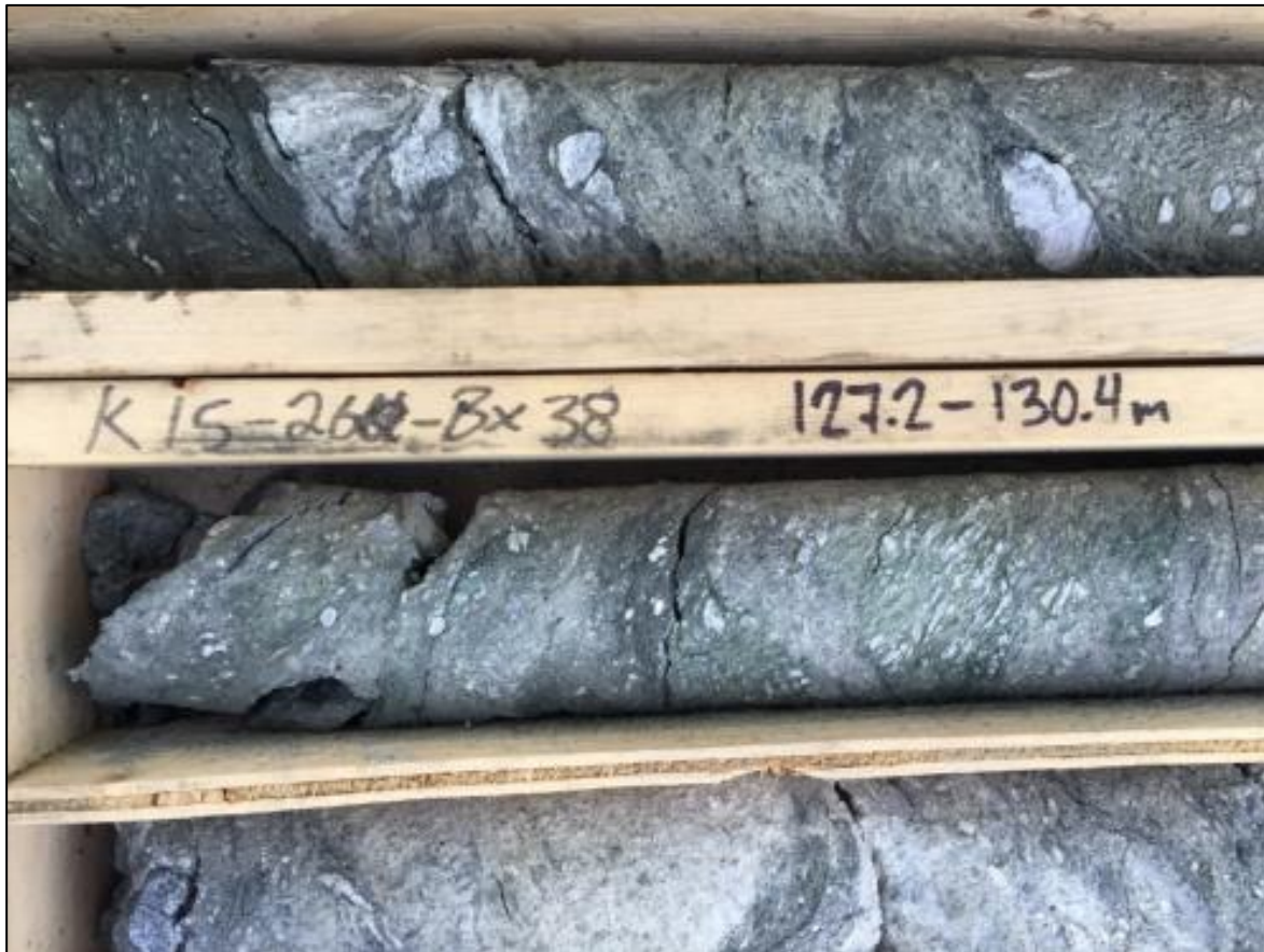
Figure 7-10: East Fault characterized by polythitic fault breccia and minor gouge (K15-262 at approximately 127.2 m) Source: Hughes and Baknes, 2015
