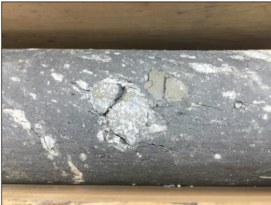
Figure 7-7: Angular to sub-rounded primary sulphide and sulphidized clasts within East Fault breccia (hole K15-292) Source: Green, 2015b
