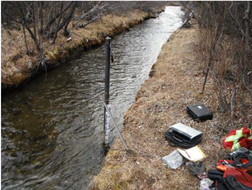
Photo 3-1: KZ-15 Hydrometric Shown as Example of Hydrometric Stations Installed at the Project
