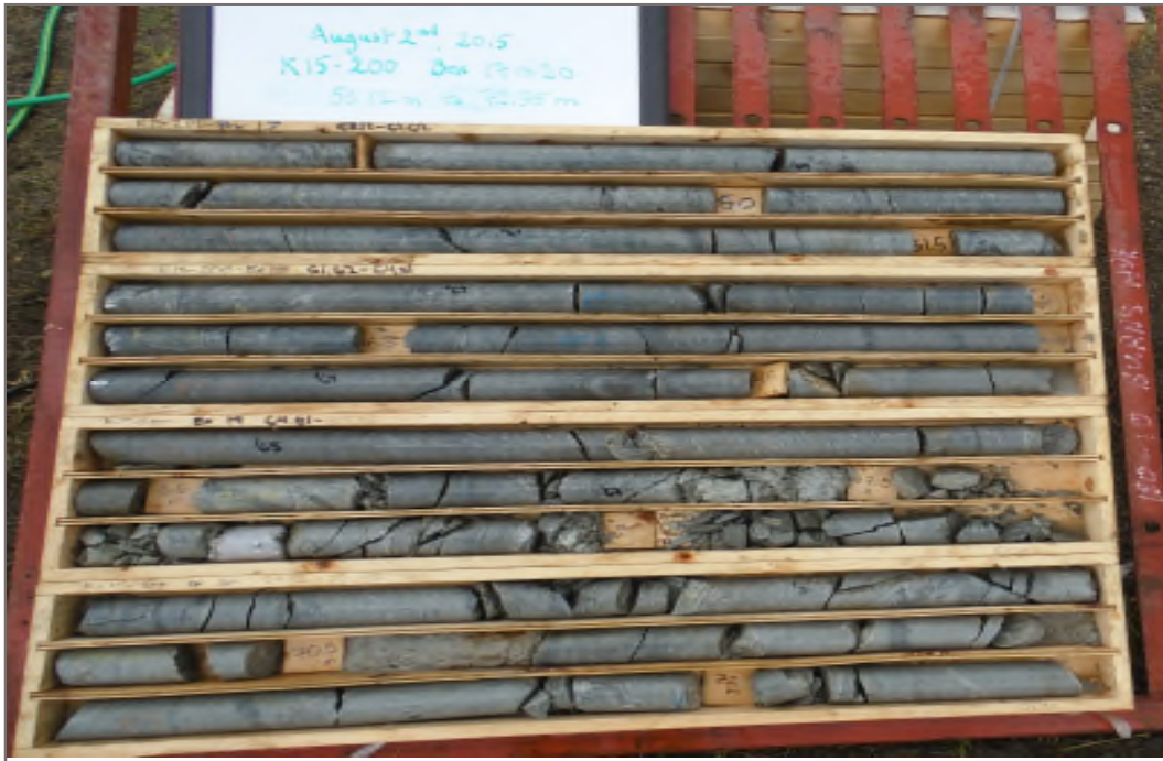
Photo 3: K15-200-WWP: 58.12 – 72.35 m ah. Packer Test #2 test interval 64.5 – 75.0 m ah.
