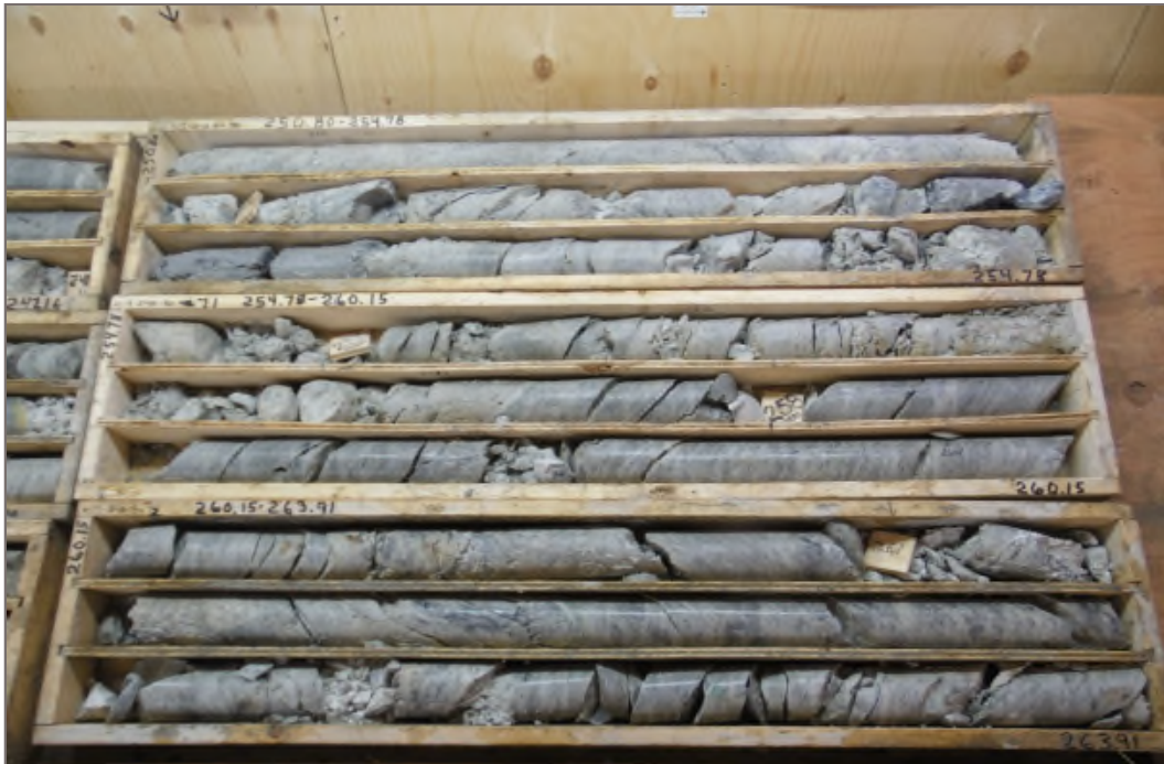
Photo 43: K15-248-WWP: 250.80 – 263.91 m ah. Packer Test #4 test interval 244.5 – 279.0 m ah.
