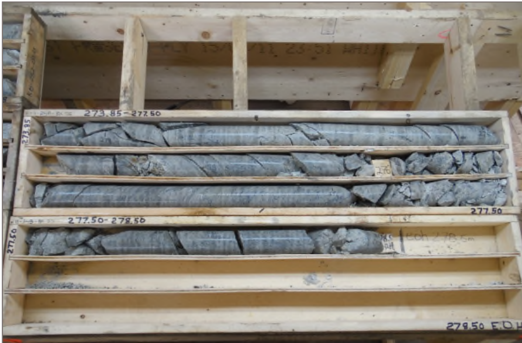
Photo 45: K15-248-WWP: 273.85 – 278.50 m ah. Packer Test #4 test interval 244.5 – 279.0 m ah.
