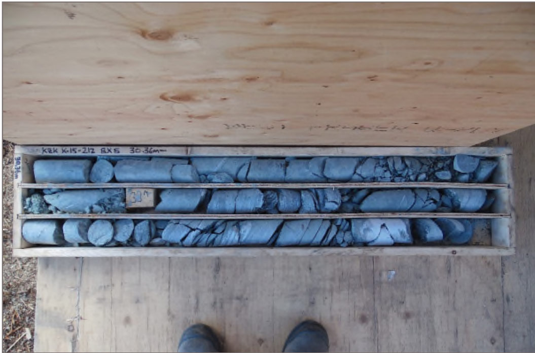
Photo 13: K15-212 / MW15-08D: 30.36 – 36.00 m bg. Well screen interval 29.8 – 35.6 m bg. Packer test interval 19.5 – 36.0 m bg.
