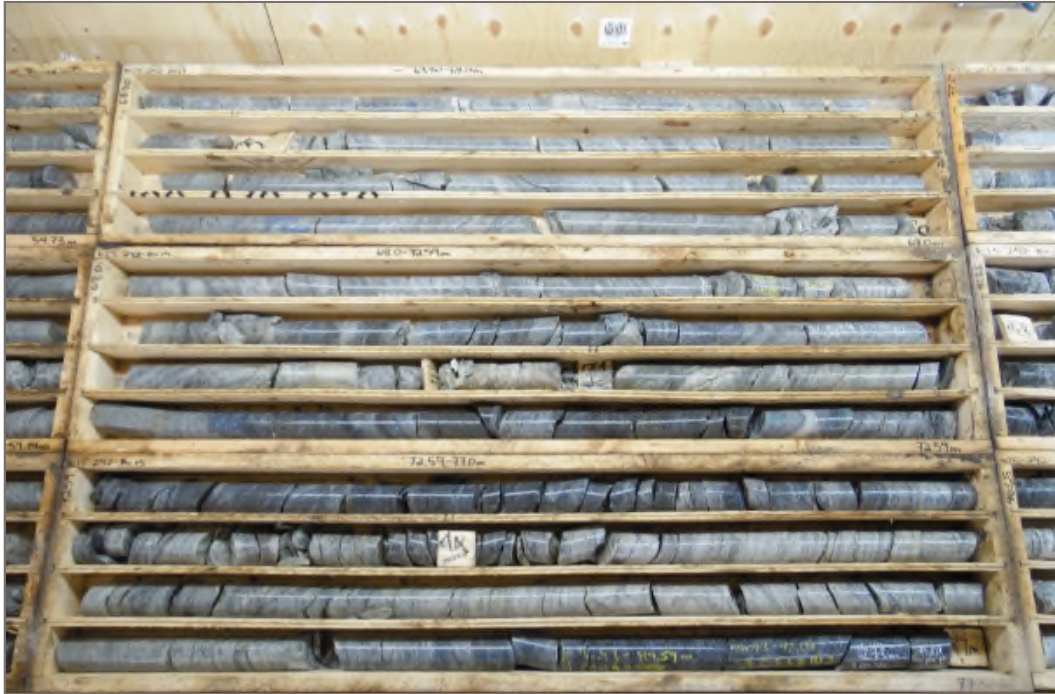
Photo 29: K15-242: 63.80 – 77.00 m ah. Packer Test #2 test interval 69.5 – 86.0 m ah.
