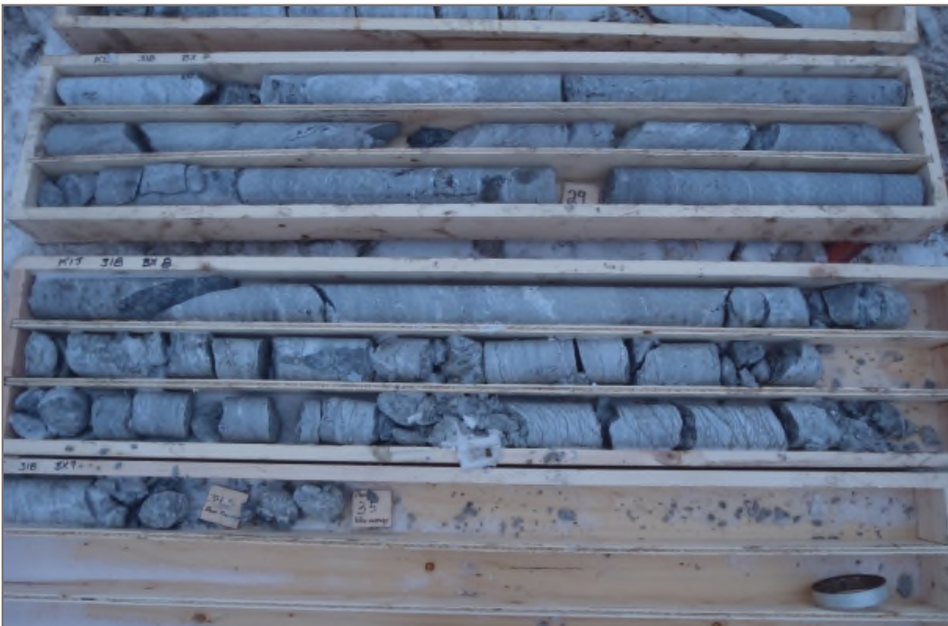
Photo 18: K15-318 / MW15-11D: ~26.25 – 35 m bg. Well screen interval 20.6 – 35.2 m bg.
