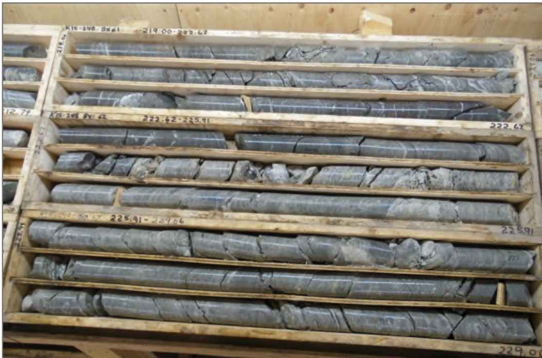
Photo 40: K15-248-WWP: 219.00 – 229.06 m ah. Packer Test #3 test interval 226.5 – 240.0 m ah.
