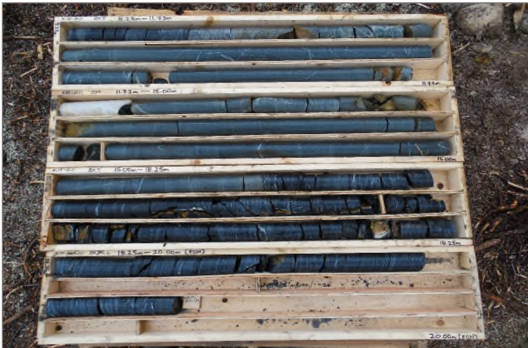
Photo 2: K15-211 / MW15-01: 8.23 – 20.00 m bg. Well screen interval 10.0 – 18.8 m bg. Packer test from 12.5 – 20.0 m bg.
