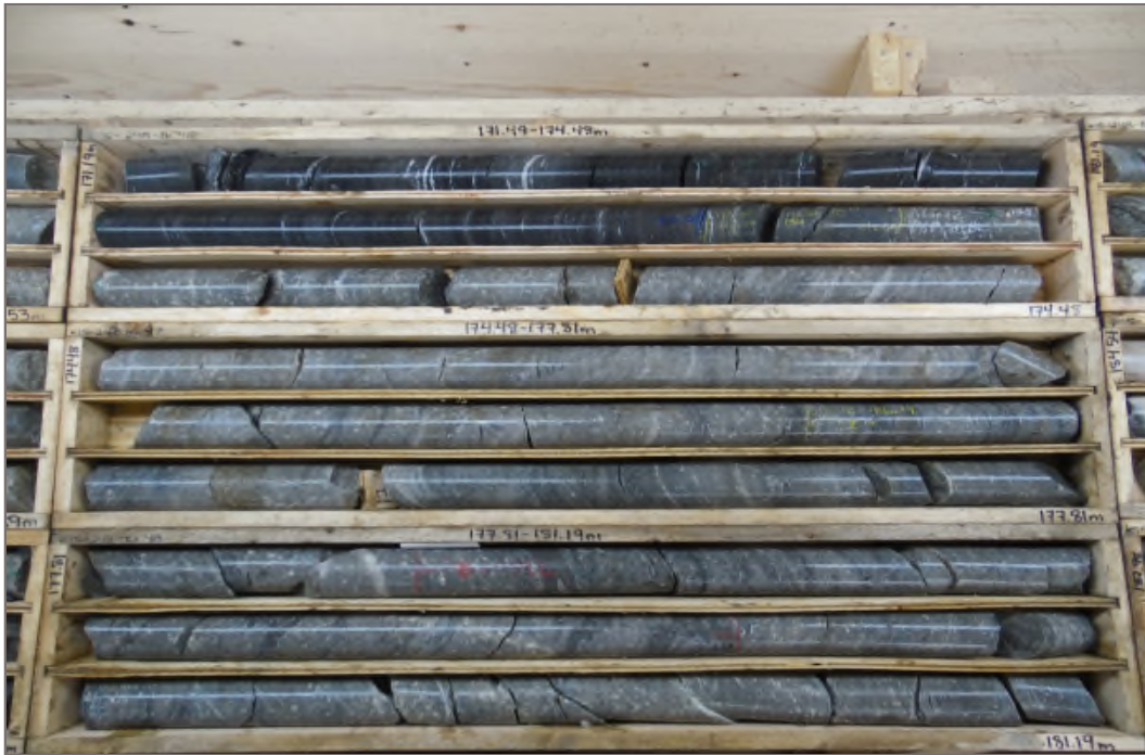
Photo 39: K15-248-WWP: 171.19 – 181.19 m ah. Packer Test #2 test interval 169.5 – 175.5 m ah.
