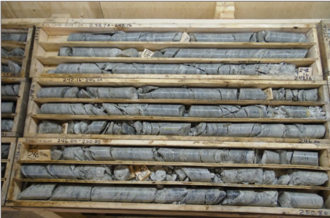
Photo 42: K15-248-WWP: 238.78 – 250.80 m ah. Packer Test #4 test interval 244.5 – 279.0 m ah.
