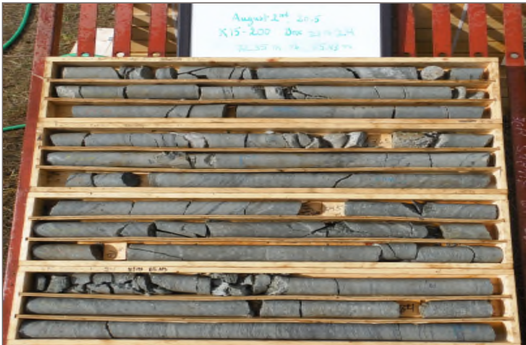
Photo 4: K15-200-WWP: 72.35 – 85.43 m ah. Packer Test #2 test interval 64.5 – 75.0 m ah.
