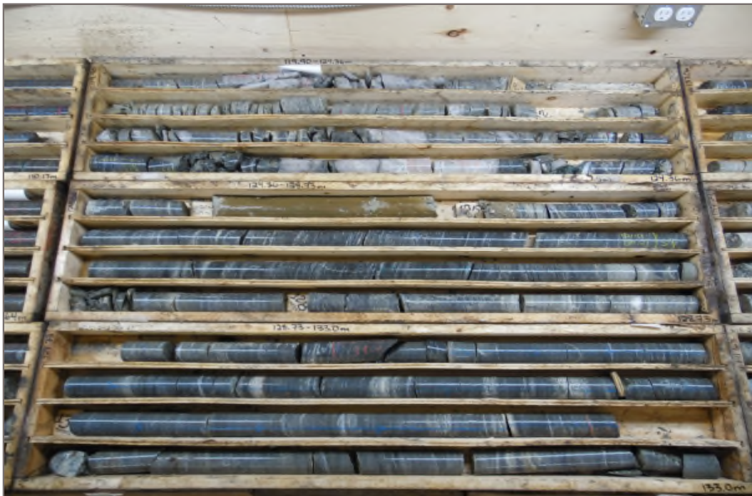
Photo 32: K15-242: 119.90 – 133.00 m ah. Packer Test #3 test interval 117.5 – 125.0 m ah and Packer Test #4 test interval 132.5 – 161.0 m ah.
