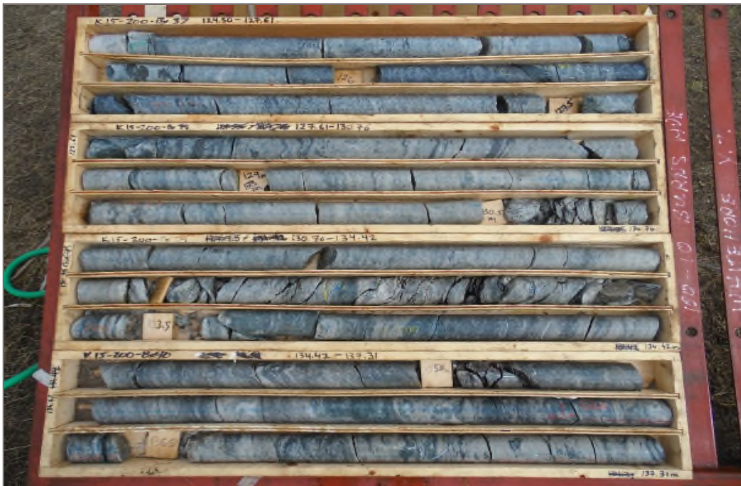
Photo 6: K15-200-WWP: 124.50 – 137.31 m ah. Packer Test #4 test interval 127.5 – 138.0 m ah.
