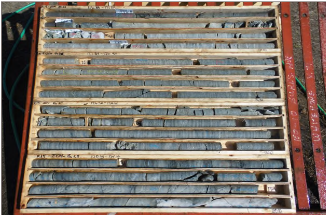
Photo 18: K15-204: 116.88 – 135.10 m ah. Packer Test #3 test interval 123.5 – 149.0 m ah.
