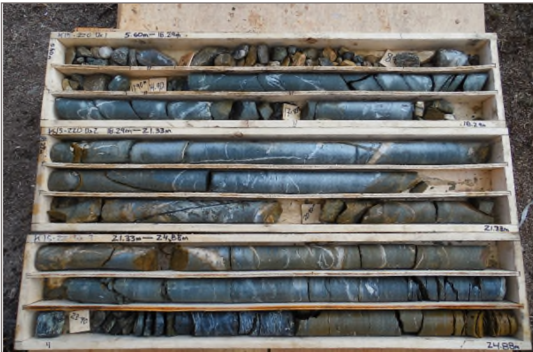
Photo 6: K15-220 / MW15-04S: 5.60 – 24.88 m bg. Well screen interval 11.2 – 14.1 m bg.
