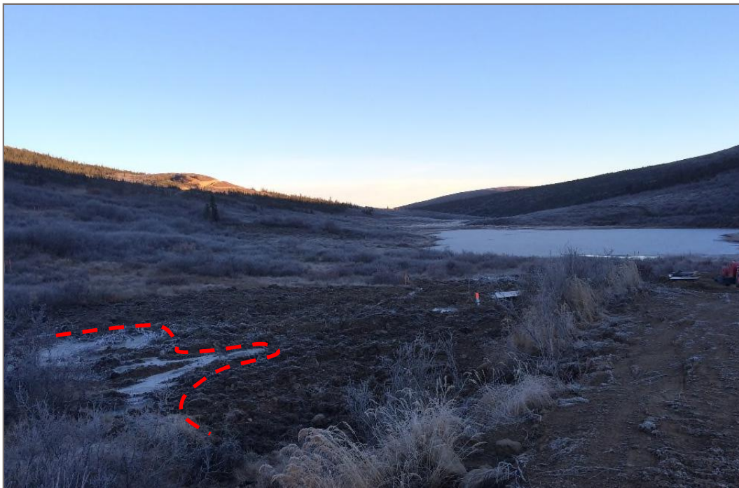
Photo 4: WW15-01 (view north) Maximum extent of overland flow (red line; approximately 50 m from surface waterbody). Water observable next to drill pipe (pipe with orange tip in centre of photograph) believed to be artesian flow from borehole and not related to pumping test program.
