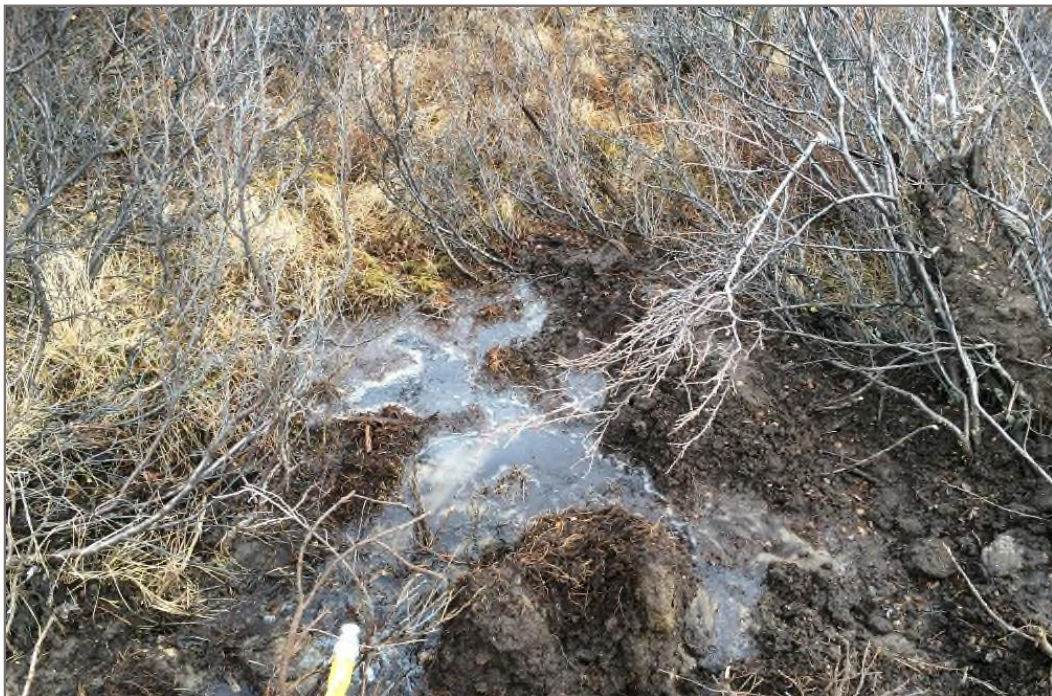
Photo 6: WW15-02, discharge to ground. After discharged water flowed under the vegetation seen at the top of this photograph, it did not daylight between this point and the creek to the east (about 200 m away).
