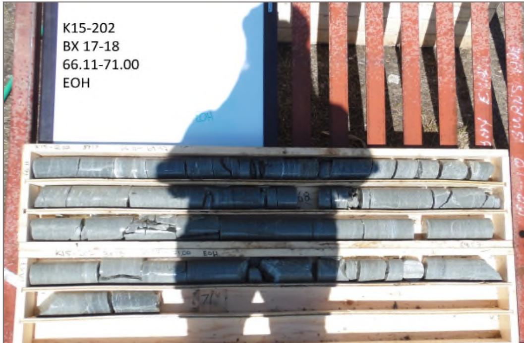
Photo 13: K15-202: 66.11 – 71.00 m ah. Packer Test #2 test interval 57.5 – 71.0 m ah.
