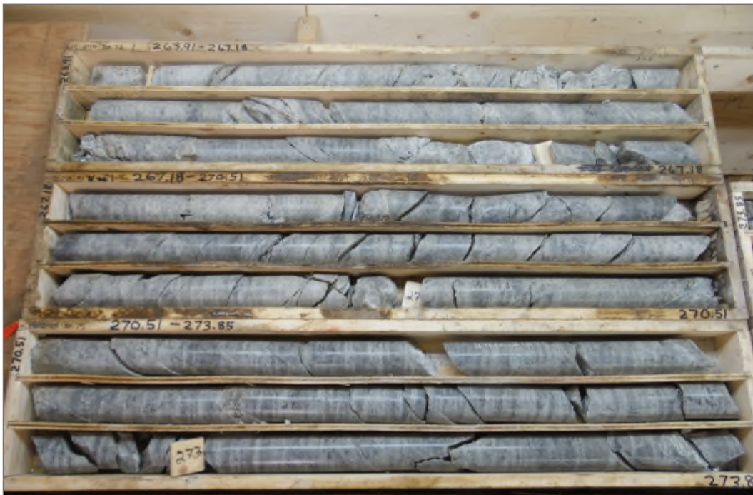
Photo 44: K15-248-WWP: 263.91 – 273.85 m ah. Packer Test #4 test interval 244.5 – 279.0 m ah.
