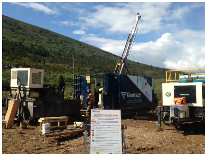
Geotech diamond drill rig at the ABM deposit. Photo taken by: Chris Hughes
