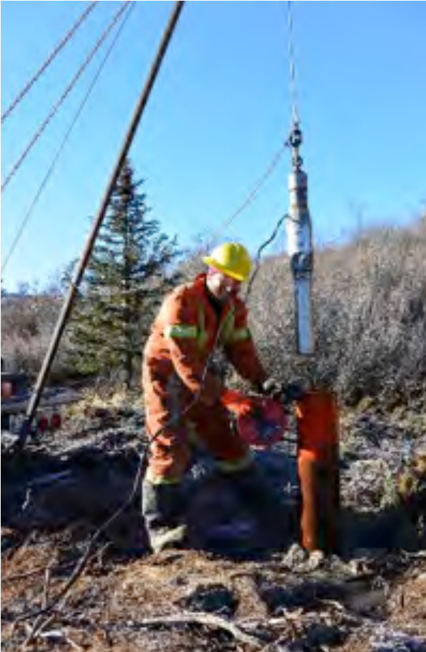
Sky Pearson initiating a pumping test
