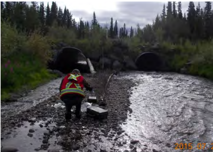
Sampling at water quality and hydrometric station (KZ-26) on Finlayson Creek near the Robert Campbell Highway. Photo taken by: Catherine Henry
