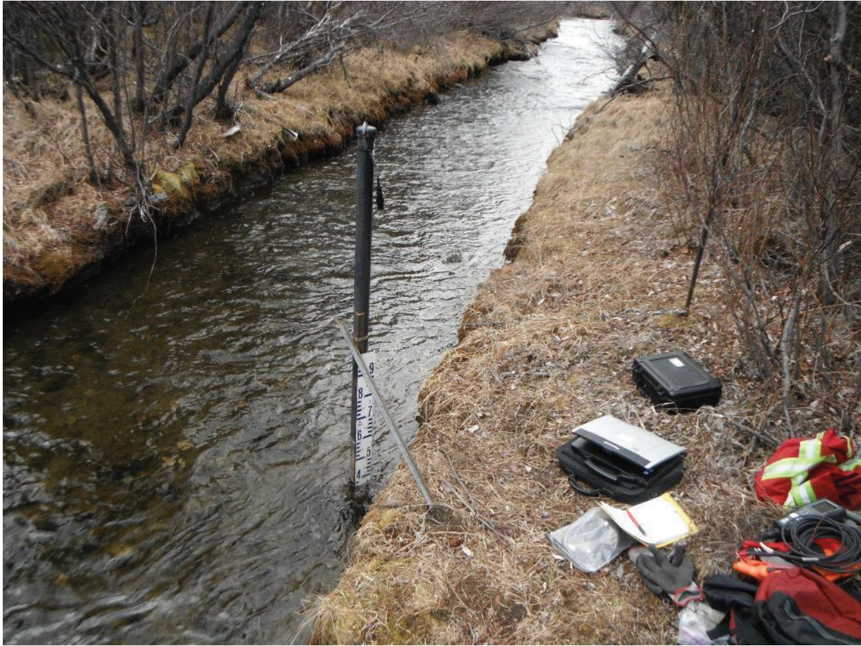
Figure 3-4: KZ-15 Hydrometric shown as example of hydrometric stations installed at the Project
