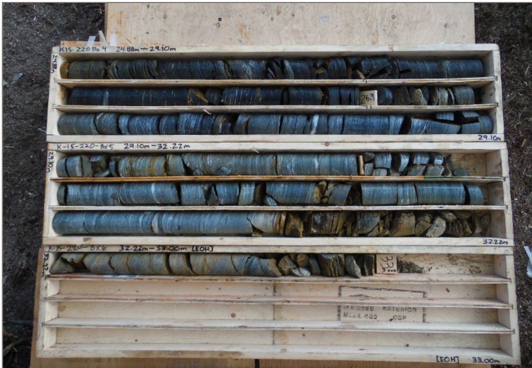
Photo 7: K15-220 / MW15-04D: 24.88 – 33.00 m bg. Well screen interval 27.1 – 32.9 m bg.
