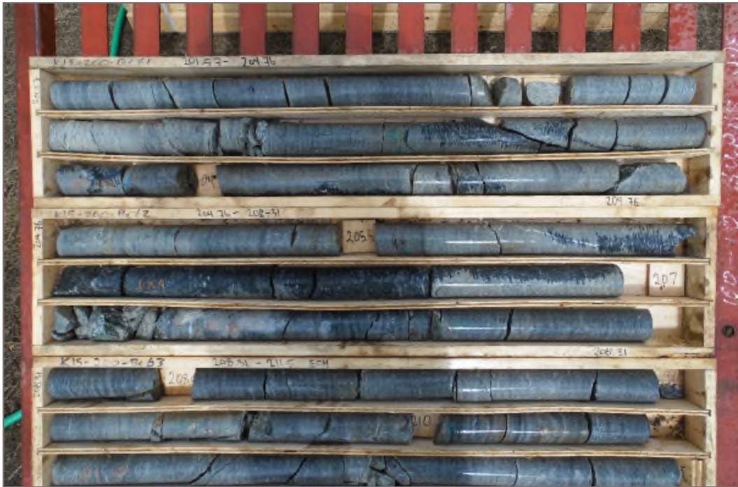
Photo 9: K15-200-WVP: 201.57 – 211.50 m ah. Packer Test #5 test interval 198.0 – 211.5 m ah.
