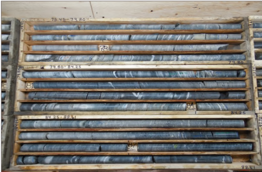
Photo 47: K15-265: 75.45 – 88.61 m ah. Packer Test #1 test interval 70.5 – 90.0 m ah.
