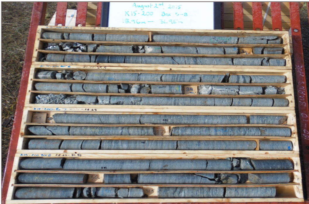
Photo 2: K15-200-WVP: 18.96 – 31.95 m ah. Packer Test #1 test interval 9.0 – 19.5 m ah.
