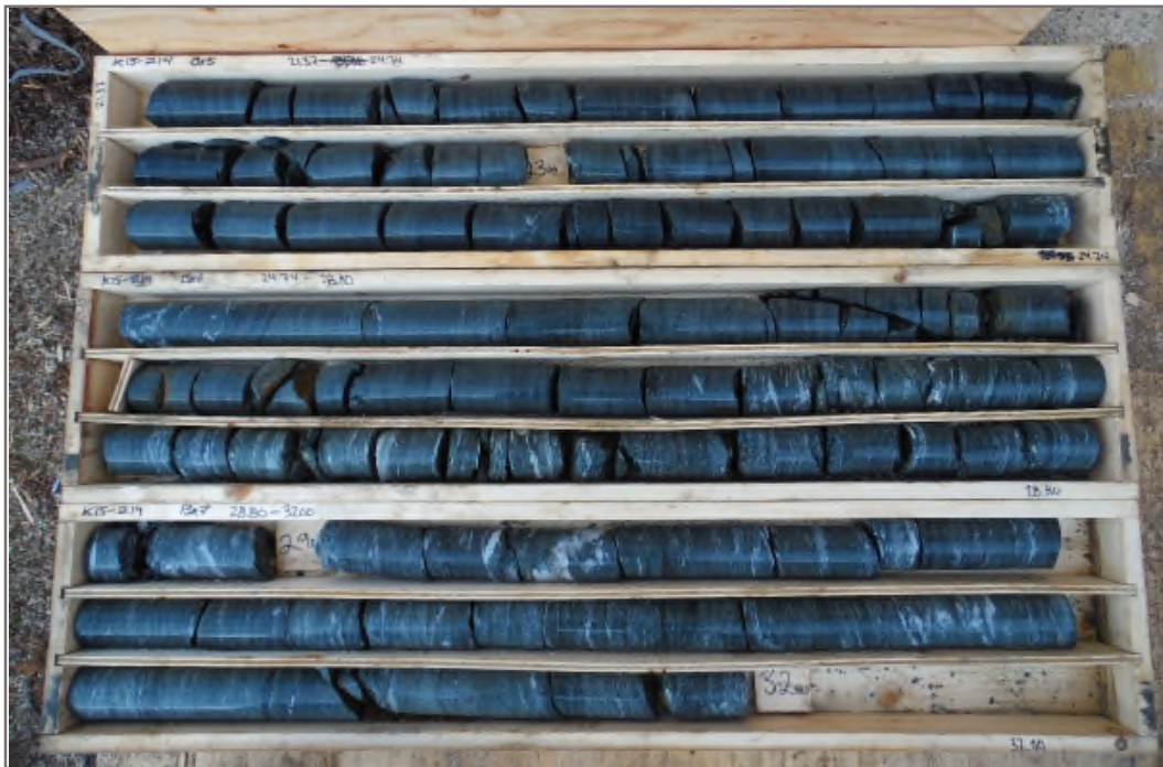
Photo 4: K15-214 / MW15-02: 21.37 – 32.00 m bg. Well screen interval 23.0 – 31.7 m bg. Packer test interval 12.5 – 32.0 m bg.
