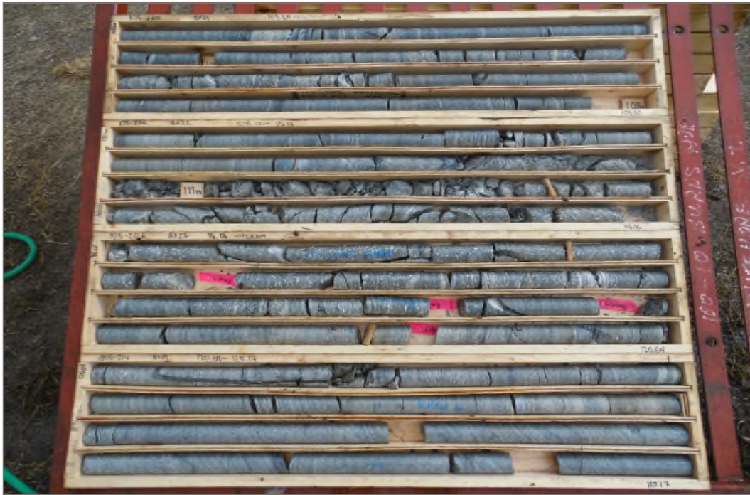
Photo 23: K15-206: 103.60 – 125.17 m ah. Packer Test #3 test interval 94.5 – 114.0 m ah.
