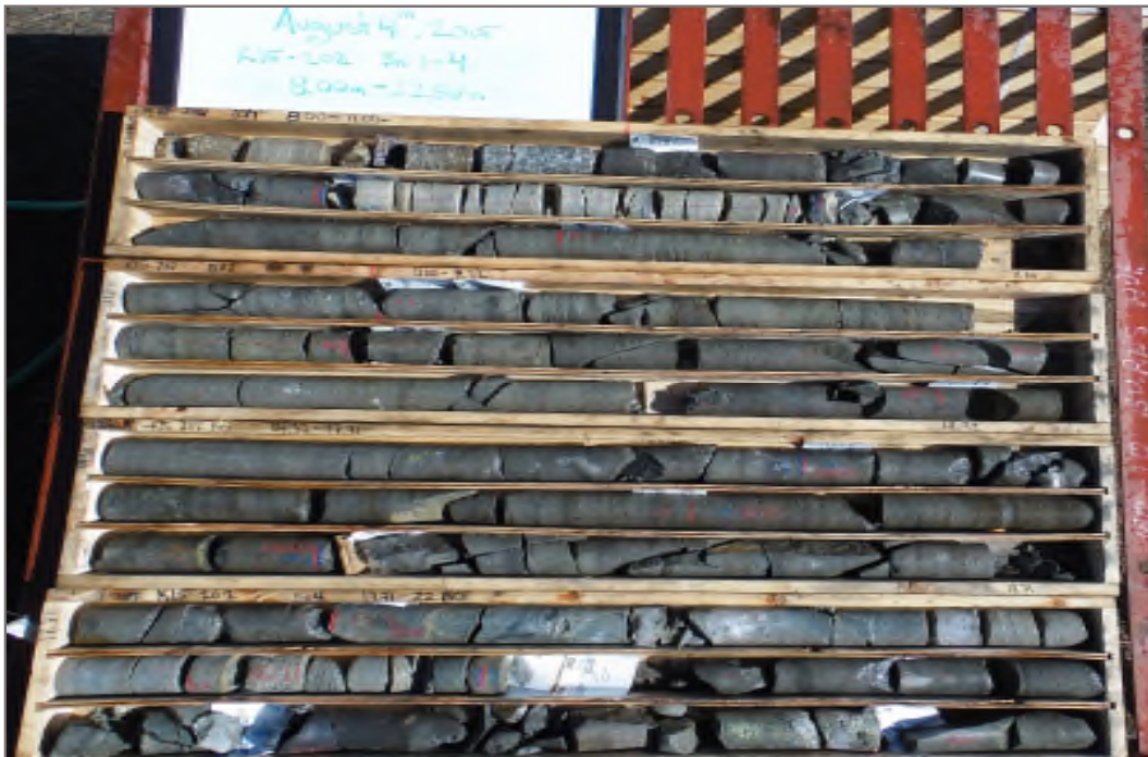
Photo 10: K15-202: 8.00 – 22.80 m ah. Packer Test #1 test interval 21.5 – 32.0 m ah.
