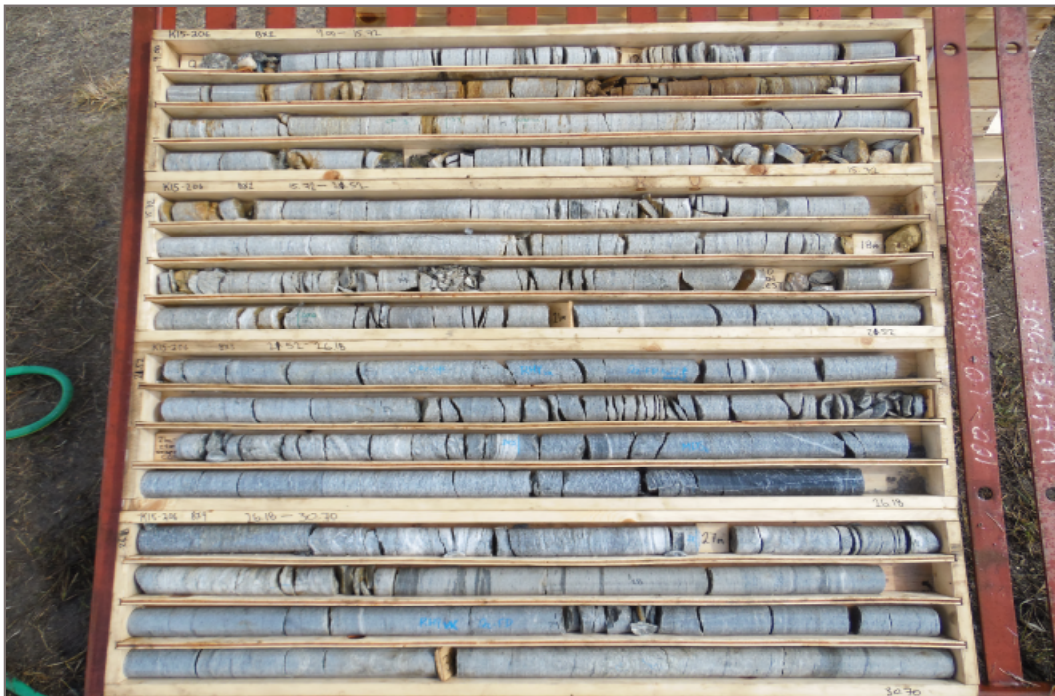
Photo 20: K15-206: 9.00 – 30.70 m ah. Packer Test #1 test interval 13.5 – 24.0 m ah.
