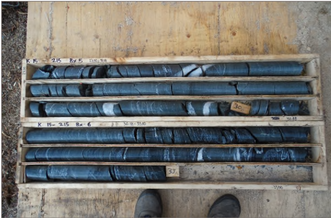
Photo 11: K15-215 / MW15-07D: 27.00 – 33.00 m bg. Well screen interval 26.3 – 32.1 m bg. Packer test interval 16.5 – 33.0 m bg.
