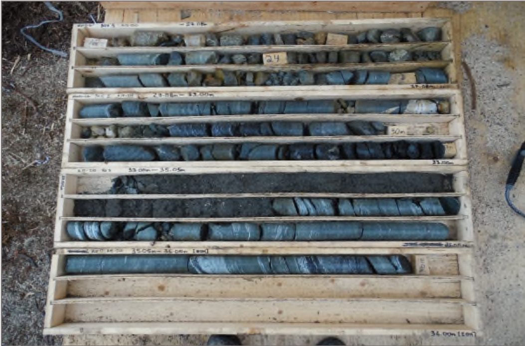
Photo 15: K15-210 / MW15-10D: 12.00 – 36.00 m bg. Well screen interval 25.7 – 31.5 m bg. Packer test interval 28.5 – 33.0 m bg.
