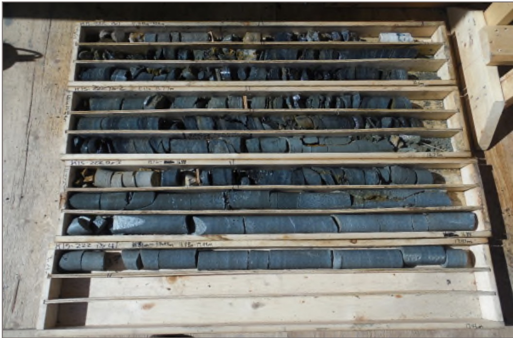
Photo 5: K15-222 / MW15-03S/D: 4.60 – 17.95 m bg. Well screen intervals 4.1 – 7.1 and 10.1 – 16.0 m bg.
