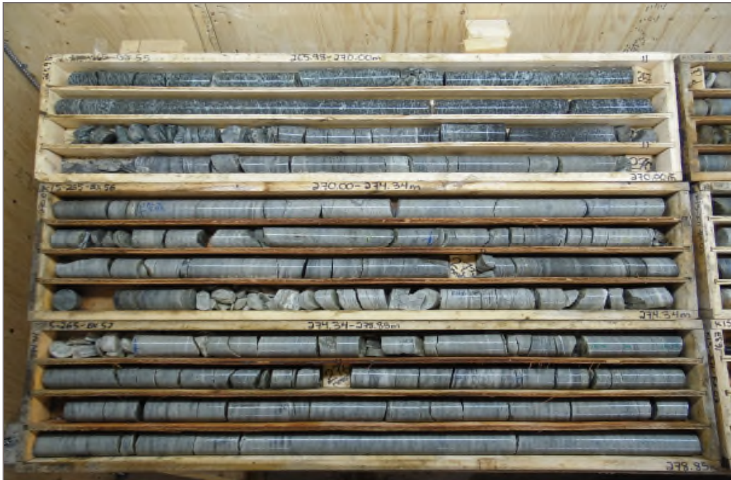
Photo 53: K15-265: 265.98 – 278.85 m ah. Packer Test #4 test interval 271.5 – 285.0 m ah.
