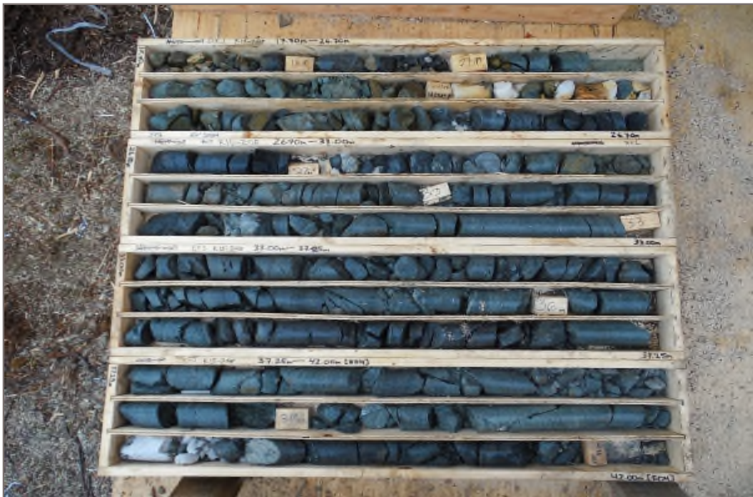
Photo 14: K15-208 / MW15-09D: 17.70 – 42.00 m bg. Well screen interval 35.1 – 40.9 m bg. Packer test interval 34.5 – 39.0 m bg.
