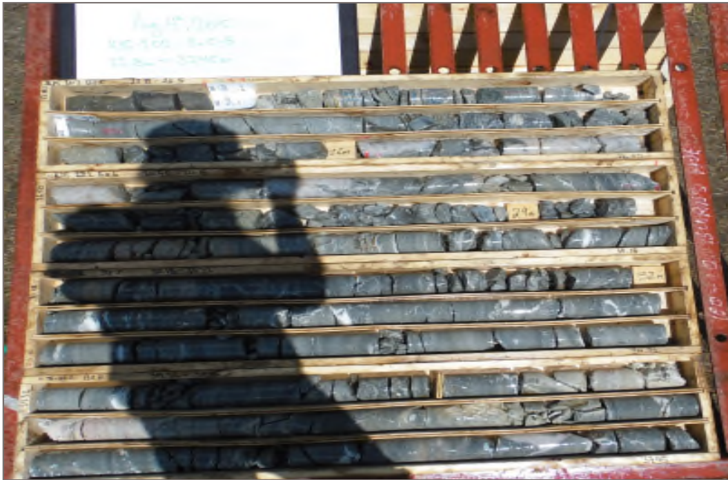
Photo 11: K15-202: 22.80 – 37.45 m ah. Packer Test #1 test interval 21.5 – 32.0 m ah.
