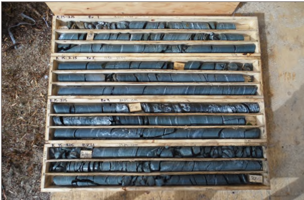
Photo 10: K15-215 / MW15-07D: 13.50 – 27.00 m bg. Well screen interval 26.3 – 32.1 m bg. Packer test interval 16.5 – 33.0 m bg.
