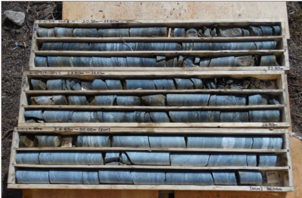
Photo 9: K15-219 / MW15-05D: 20.38 – 30.00 m bg. Well screen interval 22.4 – 29.8 m bg. Test interval 22.5 – 30.0 m bg.
