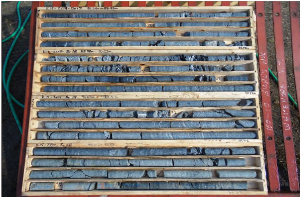
Photo 17: K15-204: 81.24 – 98.93 m ah. Packer Test #2 test interval 72.5 – 95.0 m ah.
