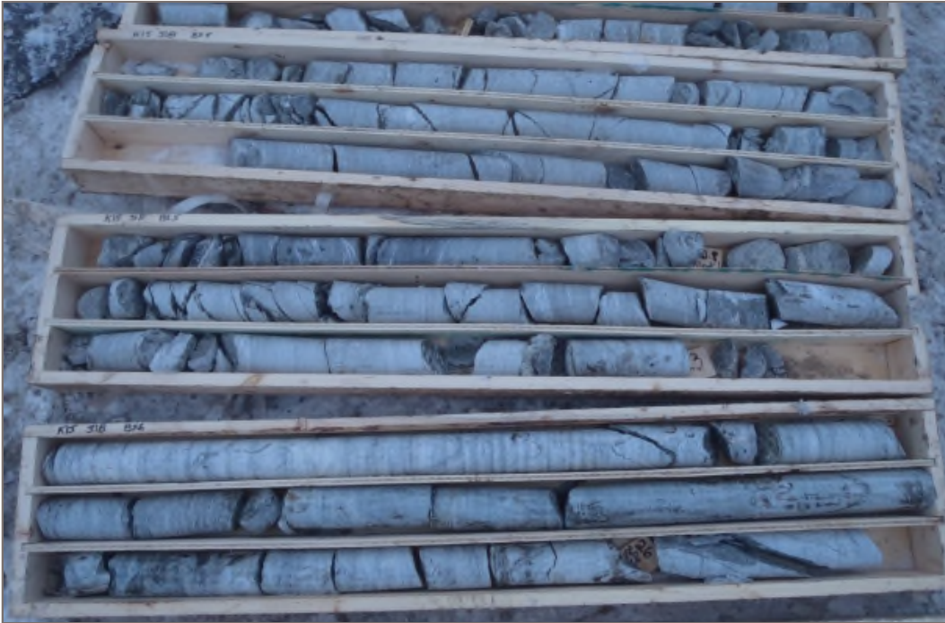
Photo 17: K15-318 / MW15-11D: ~16.95 – ~26.25 m bg. Well screen interval 20.6 – 35.2 m bg.
