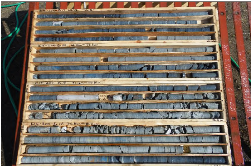
Photo 16: K15-204: 62.22 – 81.24 m ah. Packer Test #2 test interval 72.5 – 95.0 m ah.
