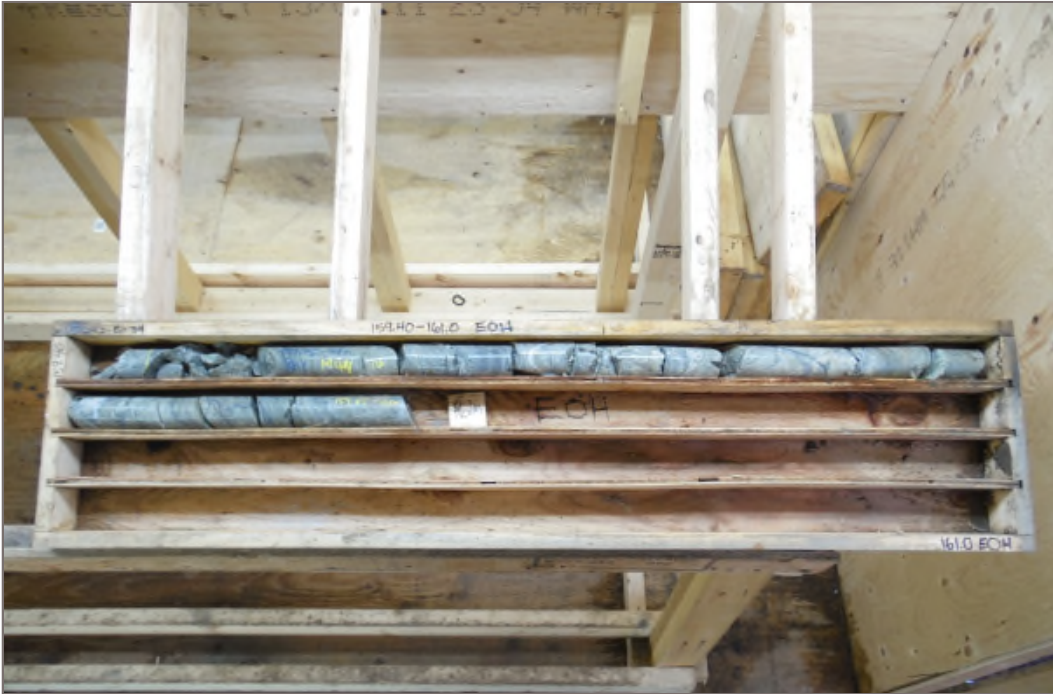
Photo 35: K15-242: 159.40 – 161.00 m ah. Packer Test #4 test interval 132.5 – 161.0 m ah.
