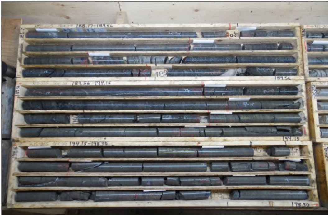
Photo 51: K15-265: 185.17 – 198.30 m ah. Packer Test #3 test interval 190.5 – 201.0 m ah.
