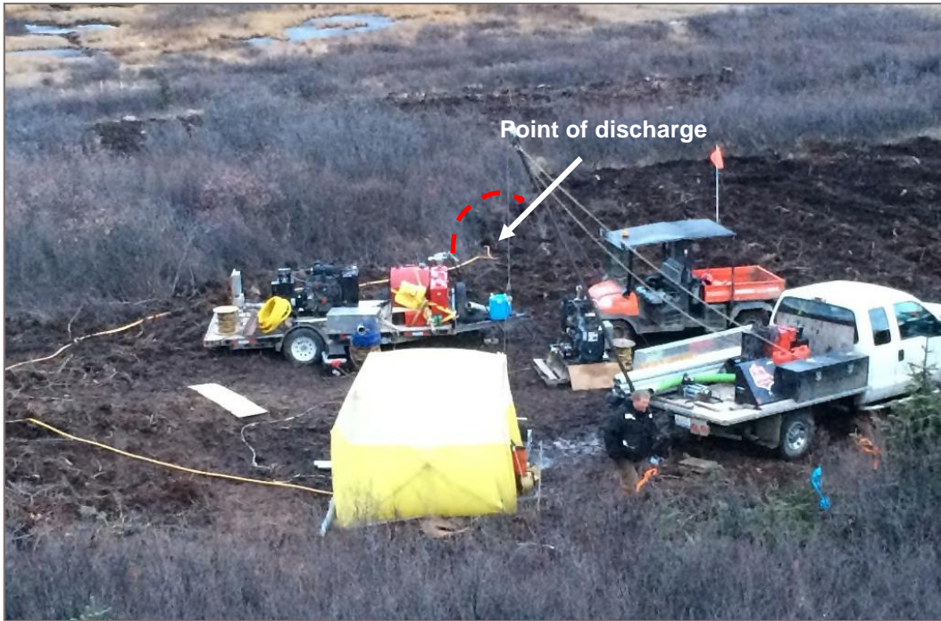
Photo 5: WW15-02 (view east) Pumping test setup, nearest surface waterbody (creek on the valley floor) is visible at the top of photograph. The red line shows the approximate extent of overland flow during water discharge.
