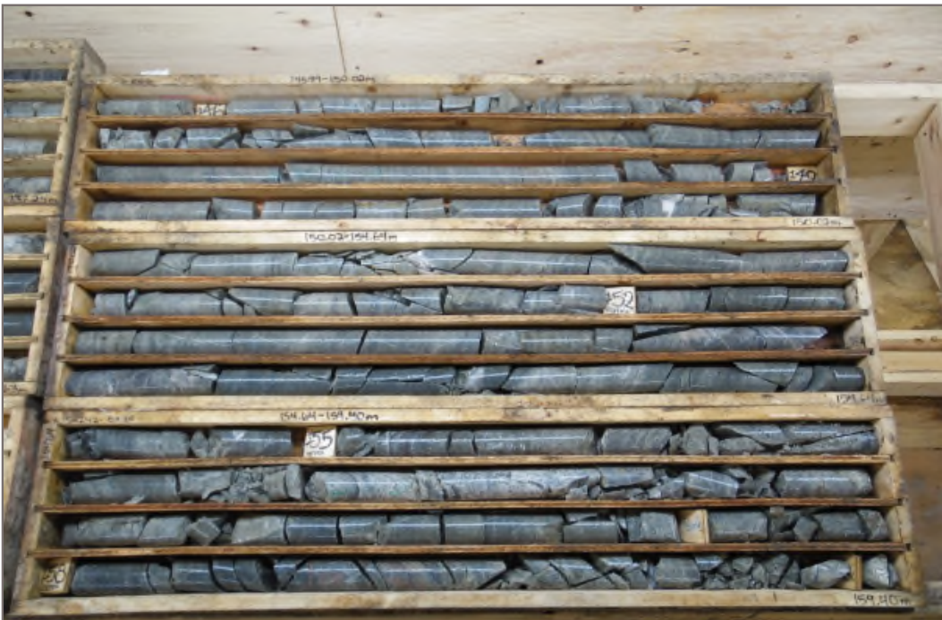
Photo 34: K15-242: 145.89 – 159.40 m ah. Packer Test #4 test interval 132.5 – 161.0 m ah.
