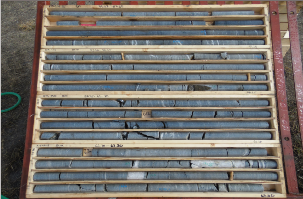
Photo 21: K15-206: 49.03 – 67.30 m ah. Packer Test #2 test interval 52.5 – 57.0 m ah.
