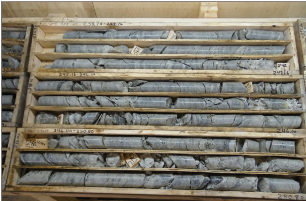
Photo 42: K15-248-WVP: 238.78 – 250.80 m ah. Packer Test #4 test interval 244.5 – 279.0 m ah.
