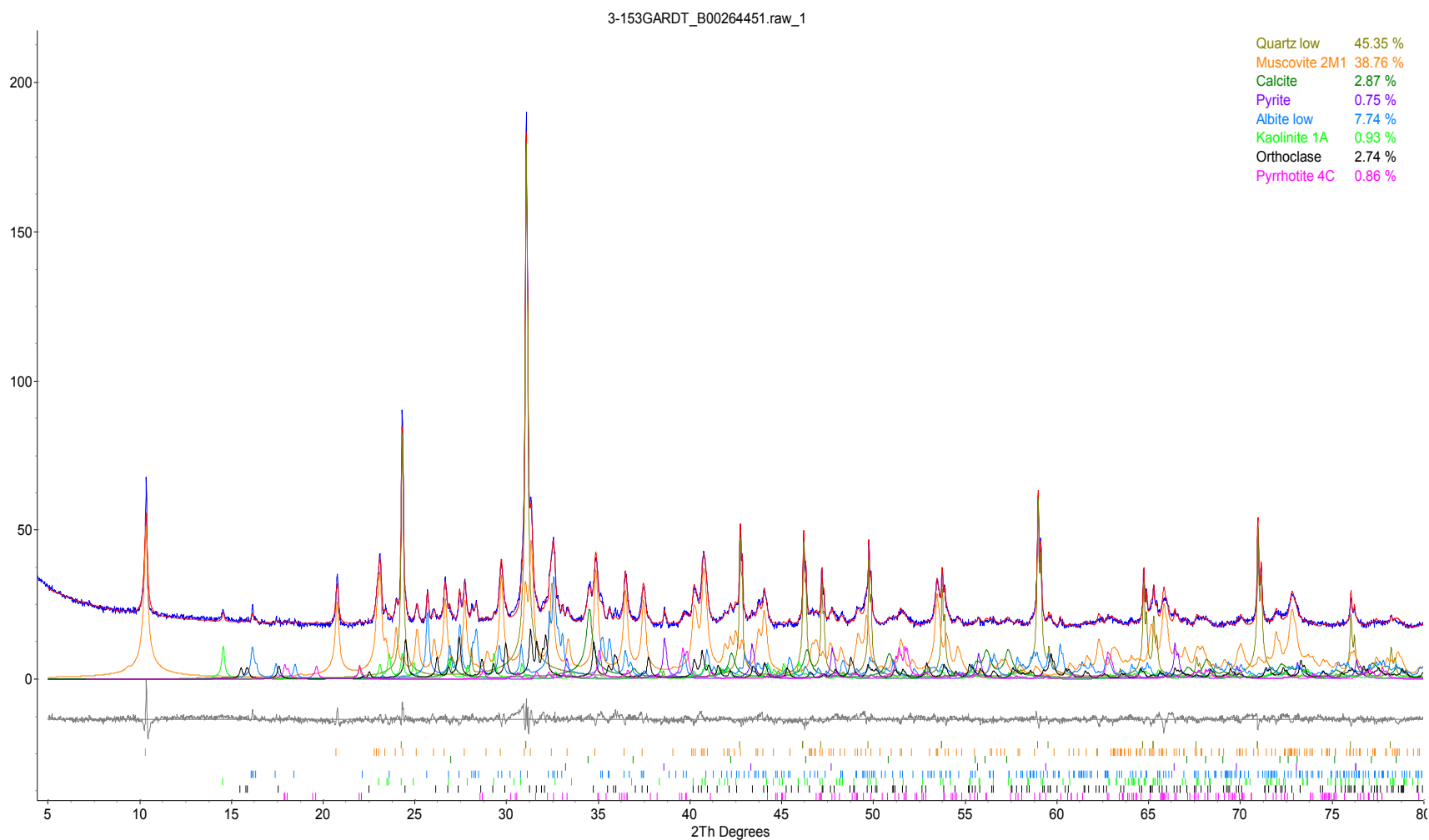
Figure 3. Rietveld refinement plot of sample Global ARD Testing Services 153: B00264451 (blue line - observed intensity at each step; red line - calculated pattern; solid grey line below – difference between observed and calculated intensities; vertical bars, positions of all Bragg reflections). Coloured lines are individual diffraction patterns of all phases.
