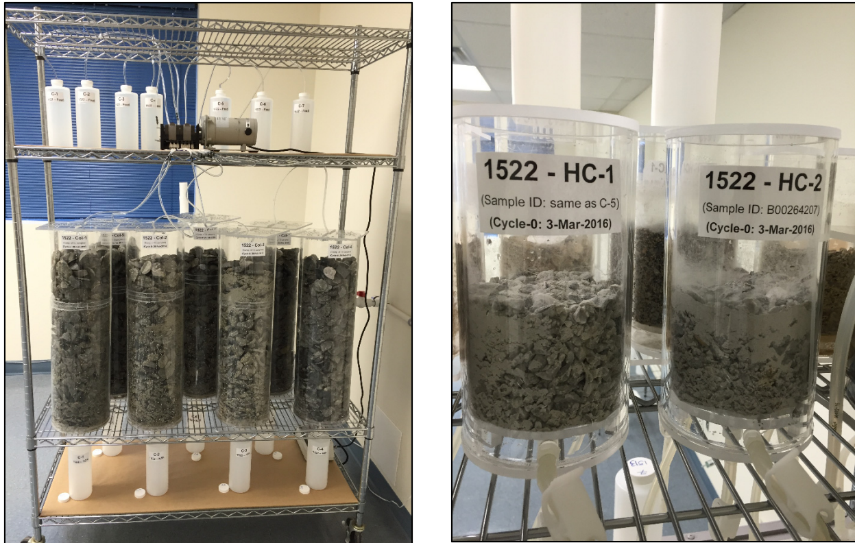
Figure 4-5: Trickle Leach Columns (left) and Humidity Cells (right) Setup
