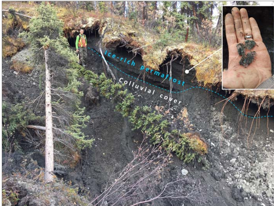
Photo 2-1. Ice-rich permafrost within till exposed in sidescarp of thermokarst gully near KM 7.5 of the existing access road to the KZK Project
