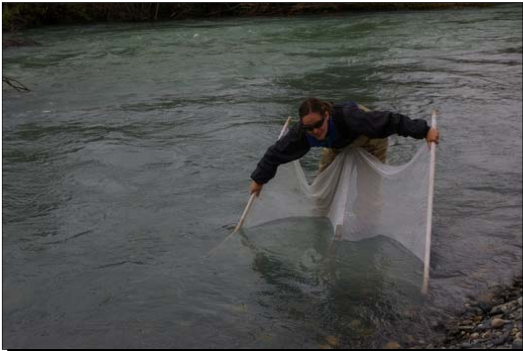
Photograph 2: A modified pole net with 3 mm mesh netting used to capture fish during electrofishing in fast currents. Photo taken August 14, 2007.
