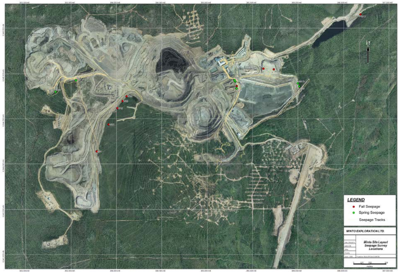
Figure 5-13: 2012 Minto Mine overview with seepage surveys (in yellow) and sample locations (fall samples in red and spring samples in green).
