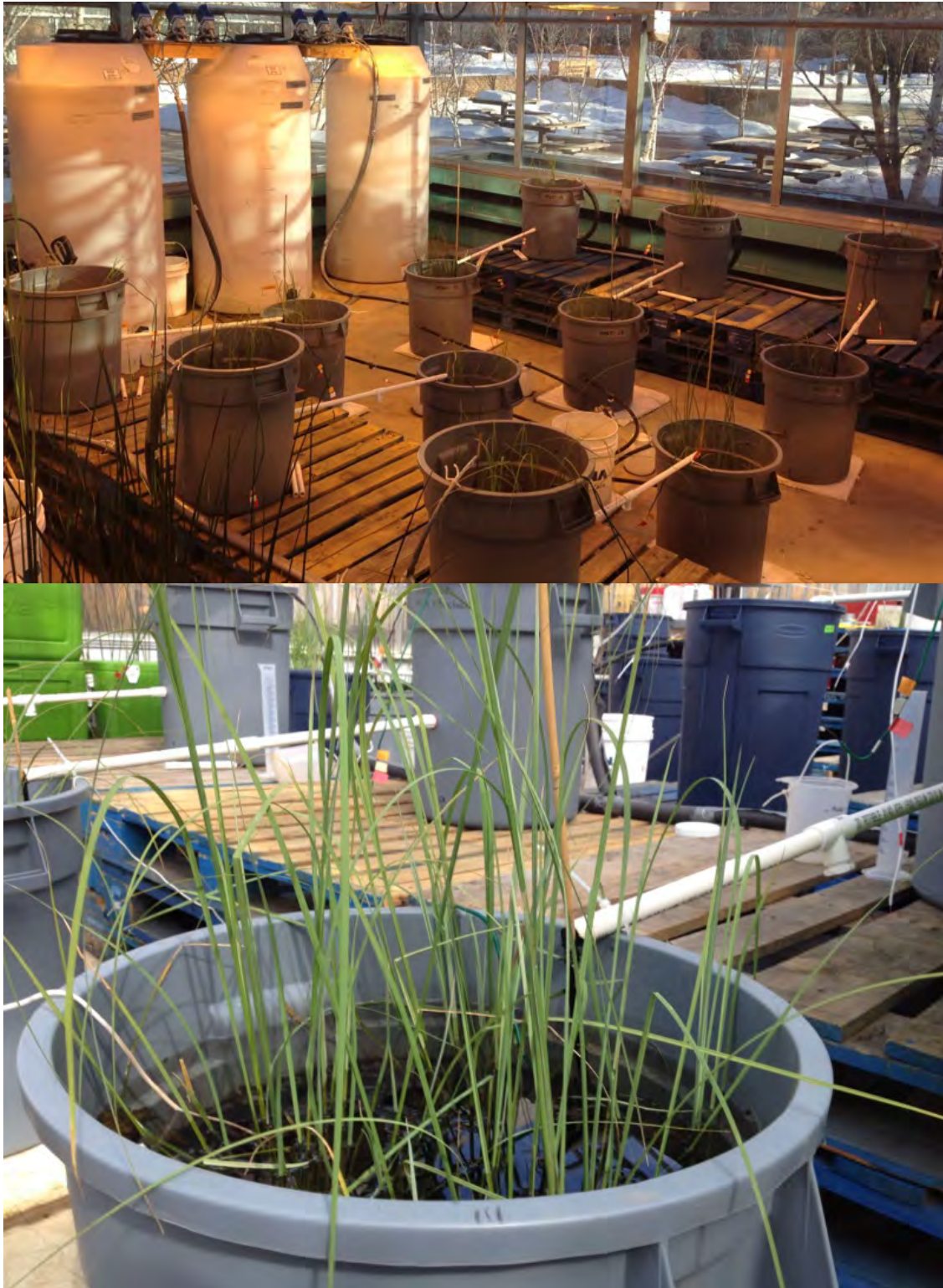
Figure 2: Photographs of pilot CWTS set up. Top is entire system, with 6 series of two cells; bottom is one cell.
