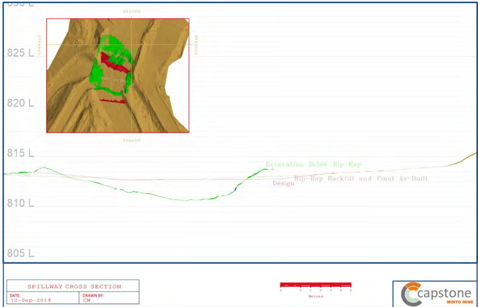
Drawing 2 – Spillway cross sectional view
