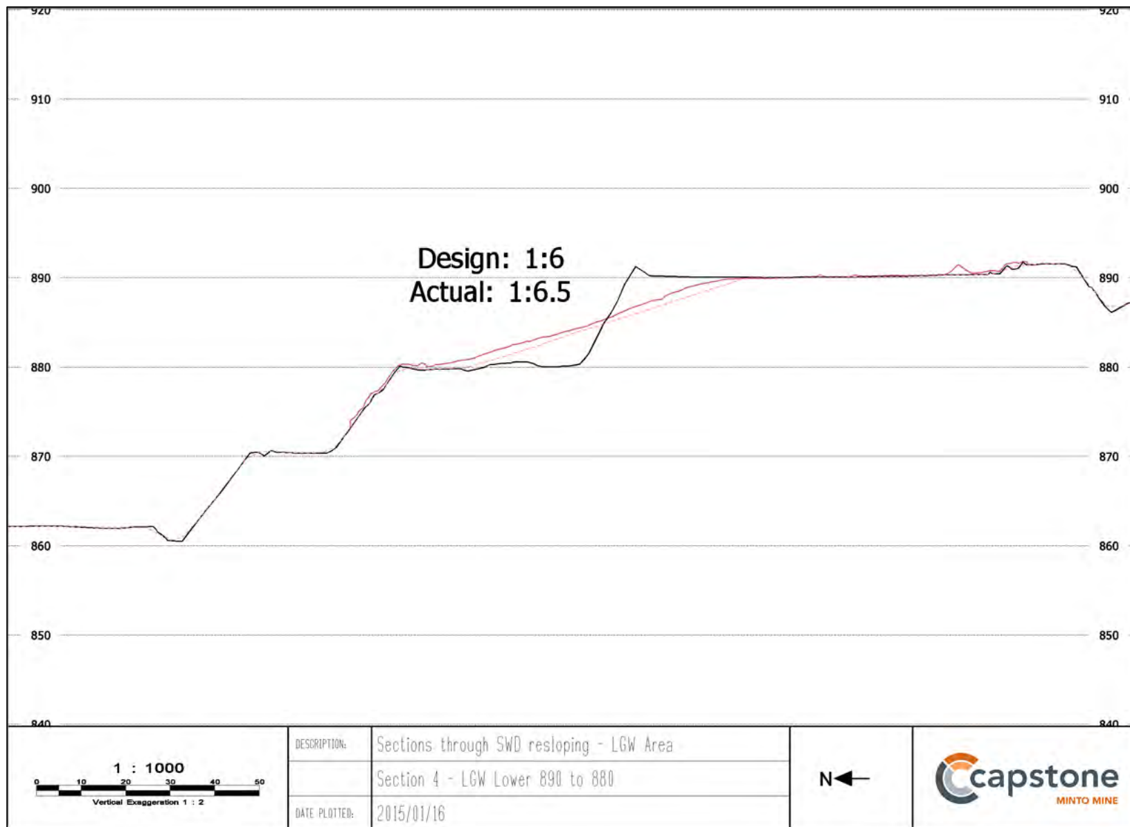
Figure 6-6: Cross Section 4 – North East Slope of the Low Grade Waste Area of the SWD
