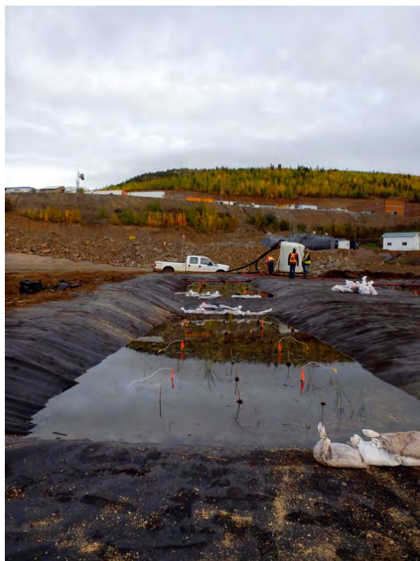
Figure 16. Series 2 (cell 2B in foreground, cell 2A in background), showing sandbags used at inflows and outflows between cells.
