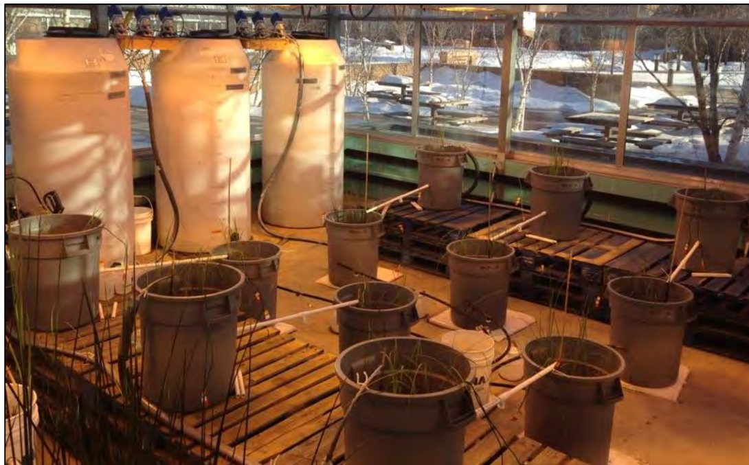
Photograph 6-2: Pilot CWTS Set Up Including Systems 1-6
