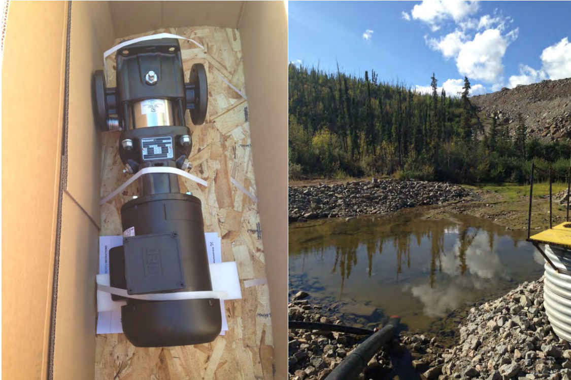
Figure 13. Water source for demonstration-scale CWTS. Left, Grundfos CR1S-6 stage pump; Right, water source at W36.
