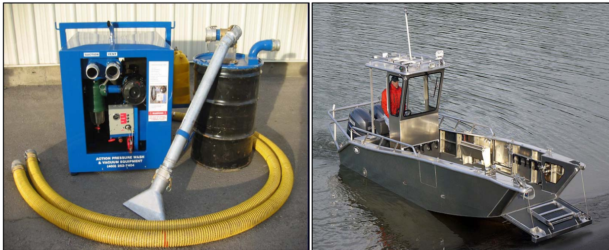
Figure 6-2: In-Viro Drum and vacuum unit and 24' Packman vessel for spill response operations
