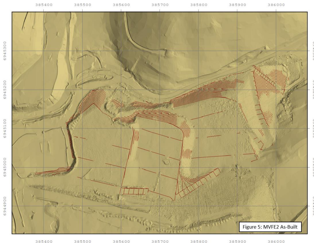
Figure 16-5: As-built surface of the Mill Valley Fill Stage 2 Extension.
