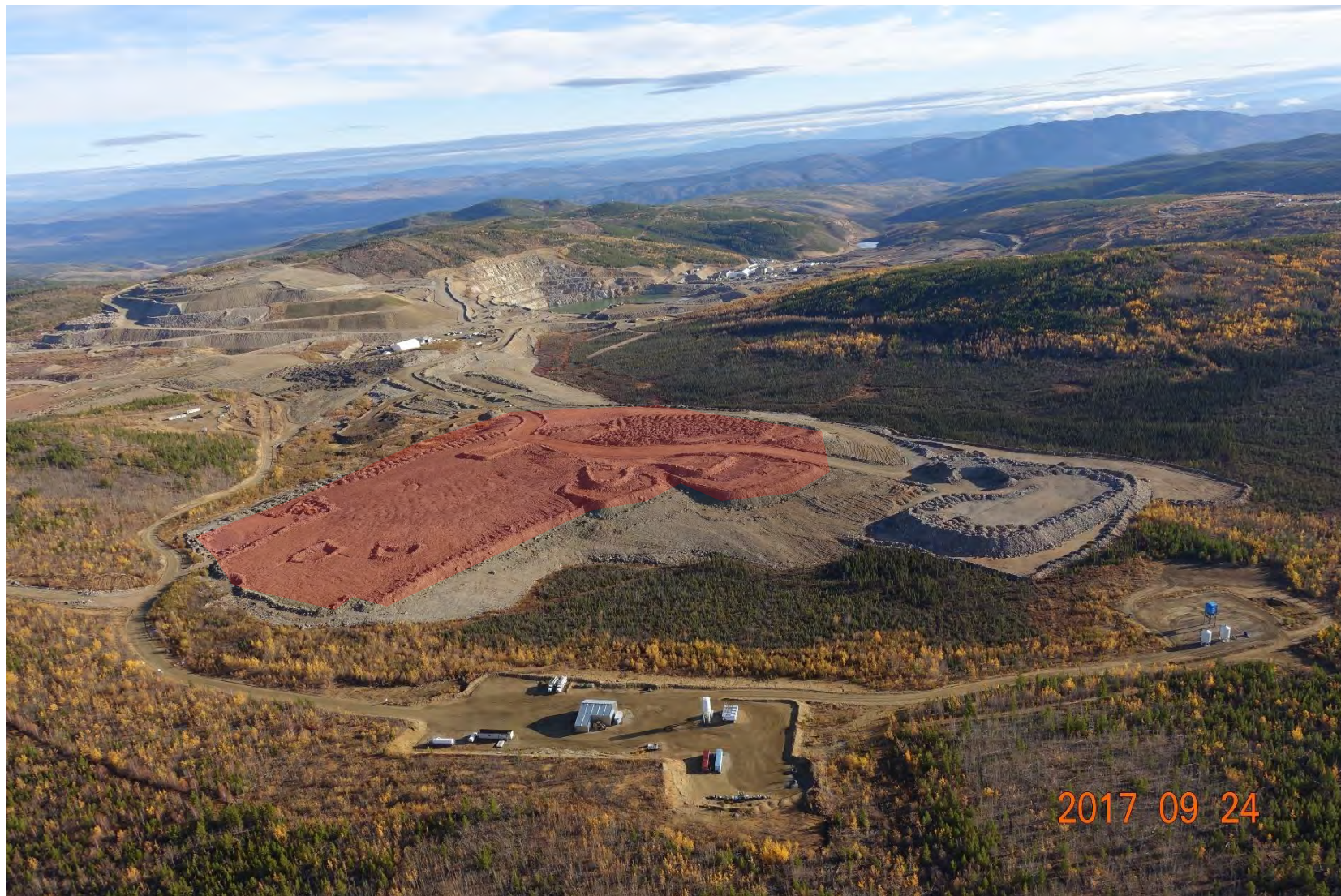
Figure 16-4: Minto Mine – Southwest dump progressive reclamation, overburden placement and stockpiling (highlighted in red).
