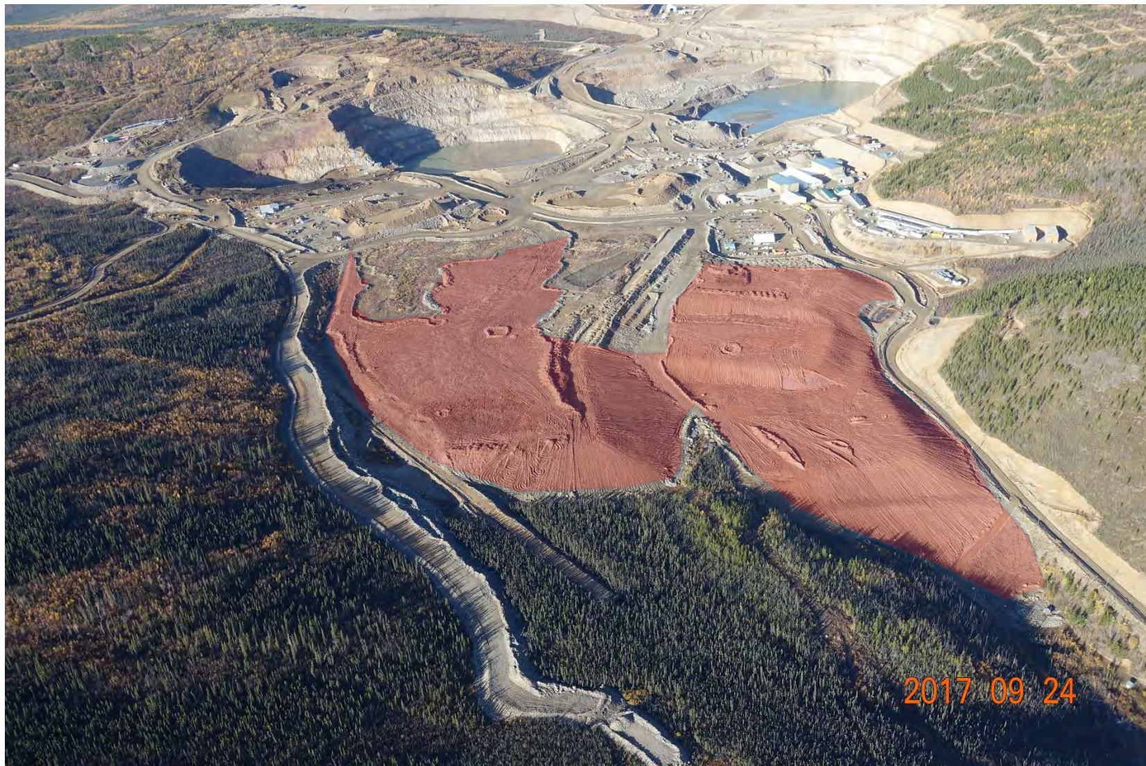
Figure 16-3: Minto Mine - MVFE and DSTSF progressive reclamation, overburden cover placement (2017 overburden placement highlighted in red).
