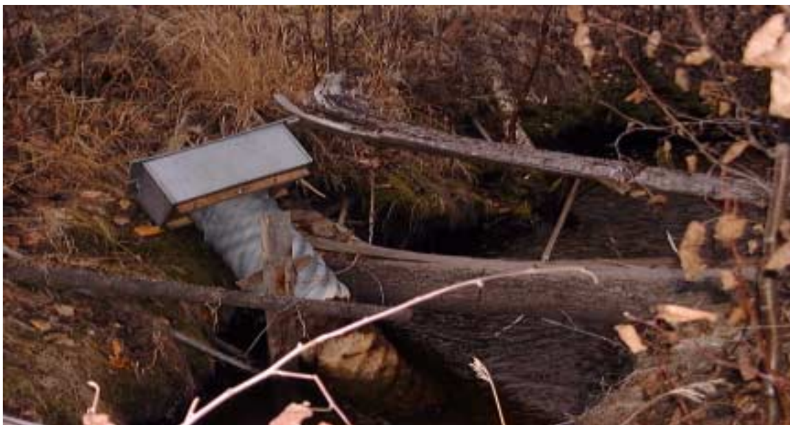
Environmental Monitoring Station W2 – Disturbed Housing for Hydrometric Datalogger
