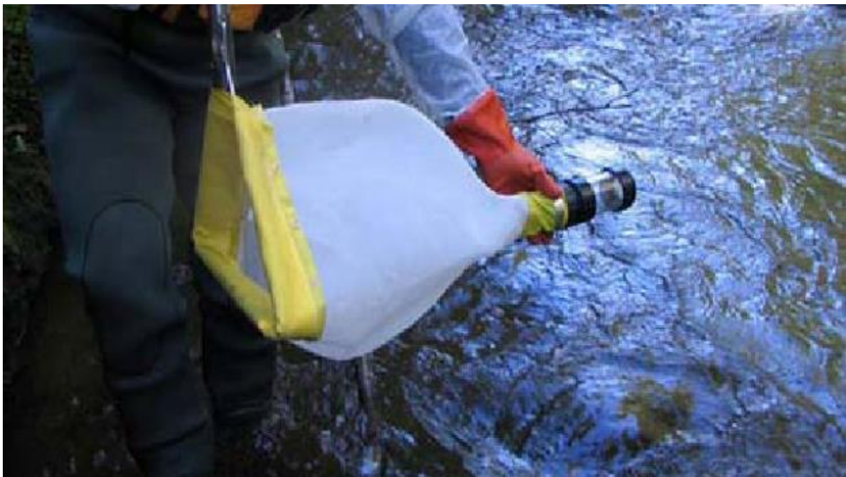
Figure 1: Kick net sampling device (Halltech Aquatic Research Inc. 2016).
