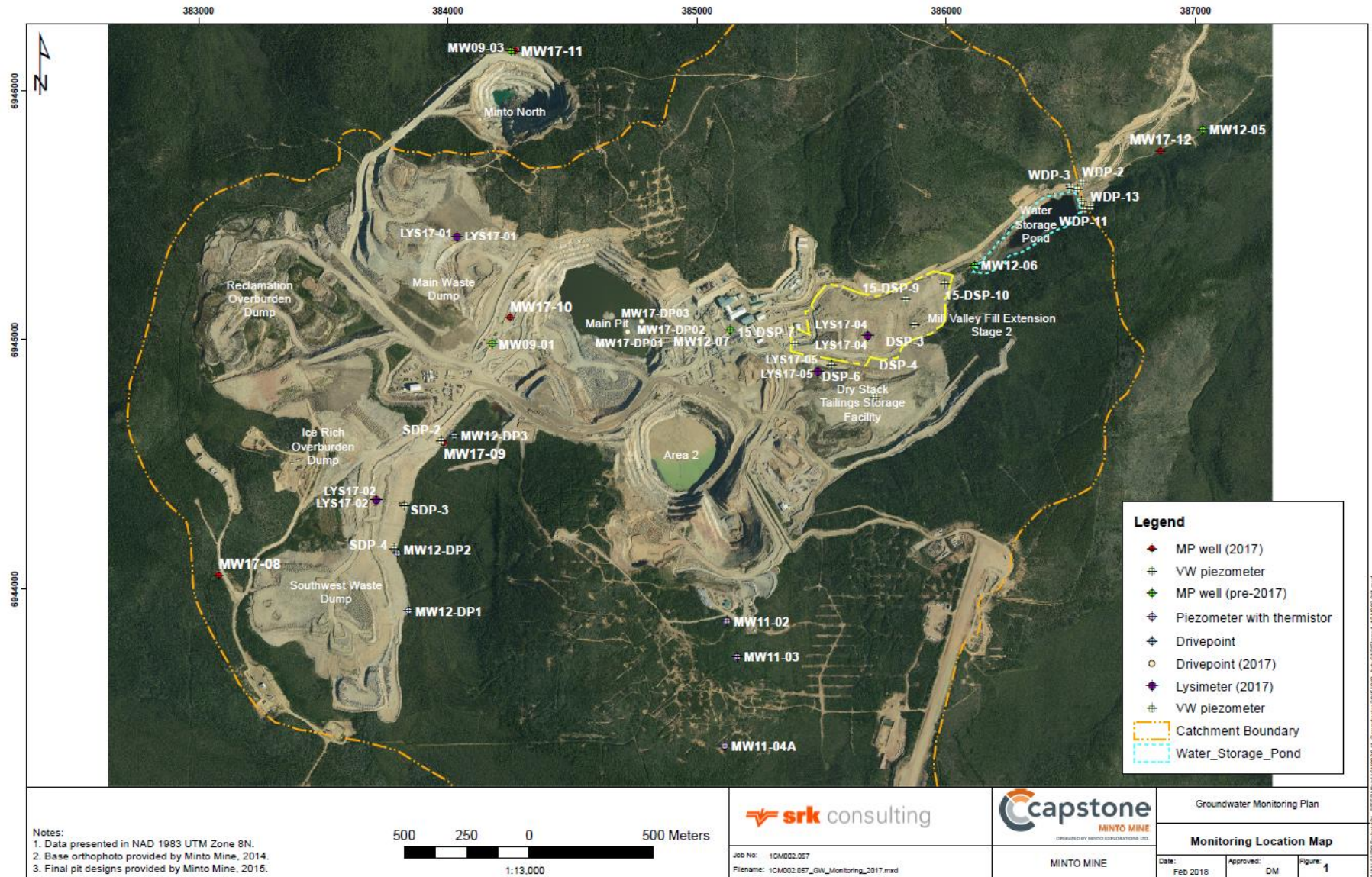
Figure 2-3: Groundwater Monitoring Site Locations
