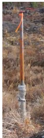
View of SWD-05A; heaved 30 cm out of the ground.
