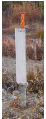
View of SWD-04A; heaved 55 cm out of the ground.
