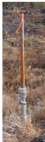
View of SWD-05A; heaved 30 cm out of the ground. (Sept. 2014 photo).
