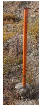
View of SWD-01A; heaved 30 cm out of the ground (Sept. 2014 photo).
