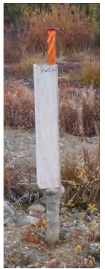
View of SWD-04A; heaved 55 cm out of the ground. (Sept. 2014 photo)
