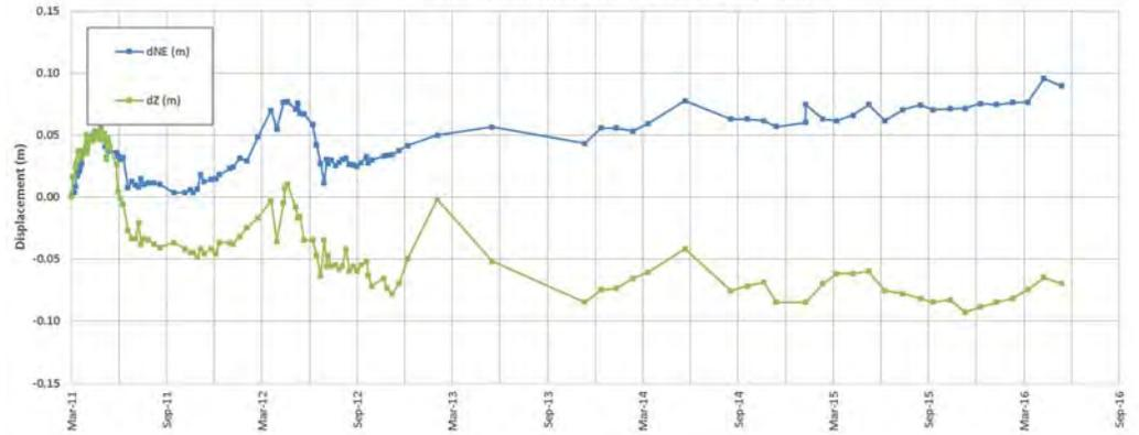
Minor movement observed at ASH06 appears to be seasonal and suspected to be related to freeze-thaw effects near the surface.
