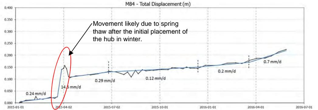
M84 - Horizontal and Vertical Displacement
