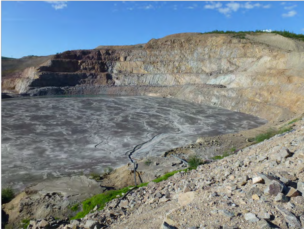
Photo 96: Area 2 Pit Stage 2 backfilled with tailings (looking south)
