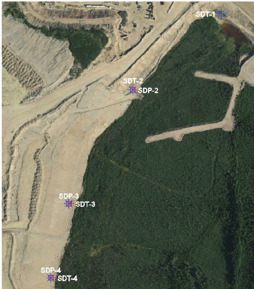
Southwest Dump Piezometers and Ground Temperature Cables
