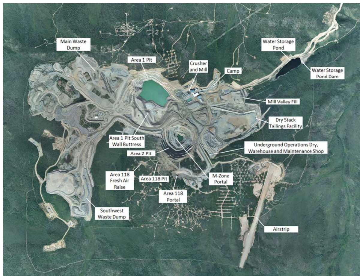
Figure 1-1: Plan view of Minto Mine (Sept. 2013) — underground and open pit operations
