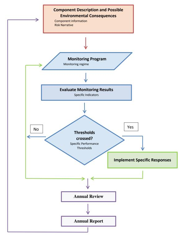
Figure 1-1: Sequential Components of the AMP (Adapted from AECOM 2010)
