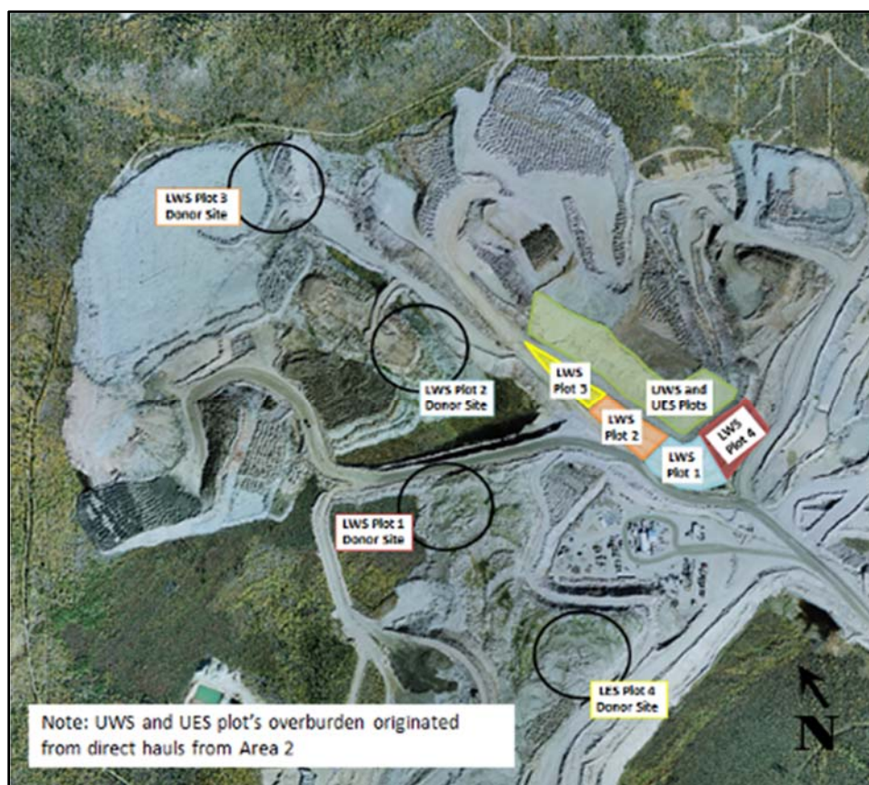
Figure 4-10 Origin of overburden material from ROD placed in distinct plots on the MWD re-contoured rock surface
