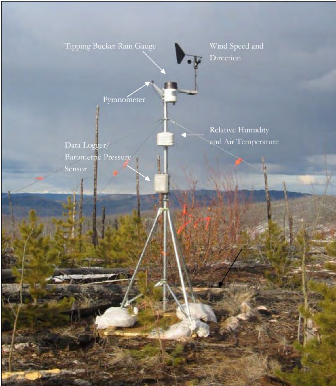
Figure 2-2: HOBO Meteorological Station at Minto (Source: EBA 2010).
