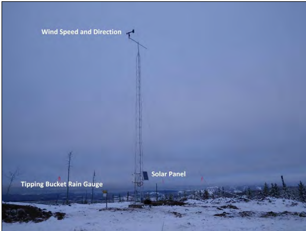
Figure 2-3: Campbell Scientific Meteorological Station at Minto.
