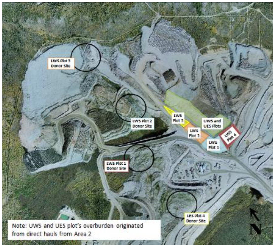
Figure 2-6: Origin of Overburden Material from ROD Placed in Distinct plots on the MWD Re-contoured Rock Surface
