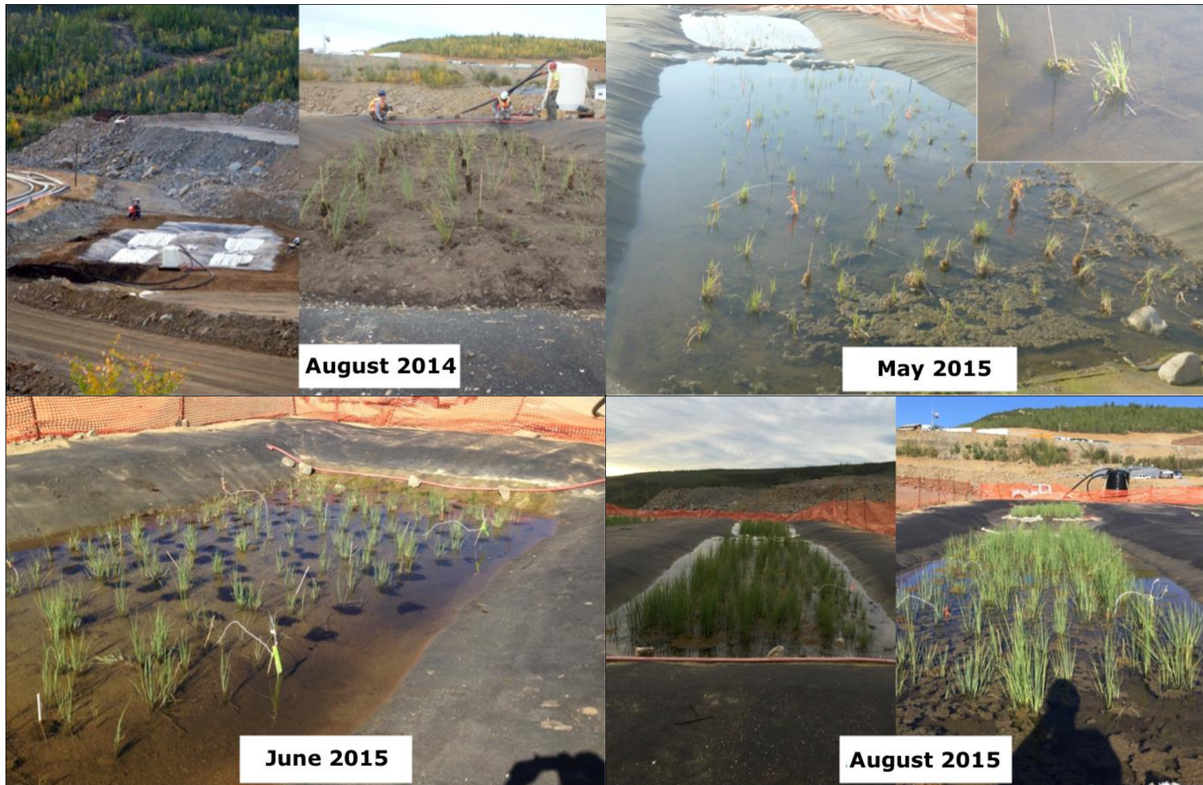
Figure 2-8: Time Lapse Photos of Demonstration Scale Treatment Wetlands at Minto Mine.
