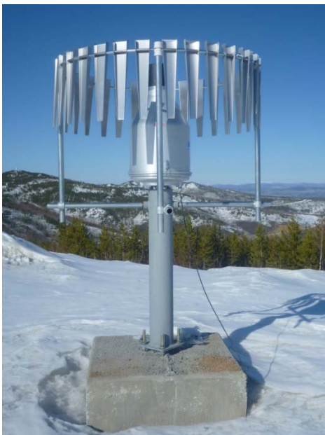
Figure 1: Minto's Geonor Precipitation Gauge
