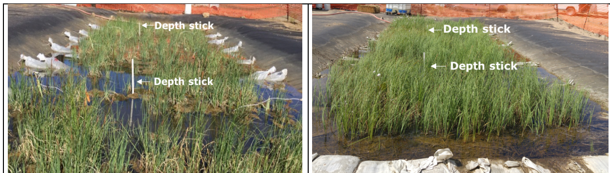
Figure A5 – Depth sticks in CWTS cell 1A to record evapotranspiration in 2016 (left) and 2017 (right).
