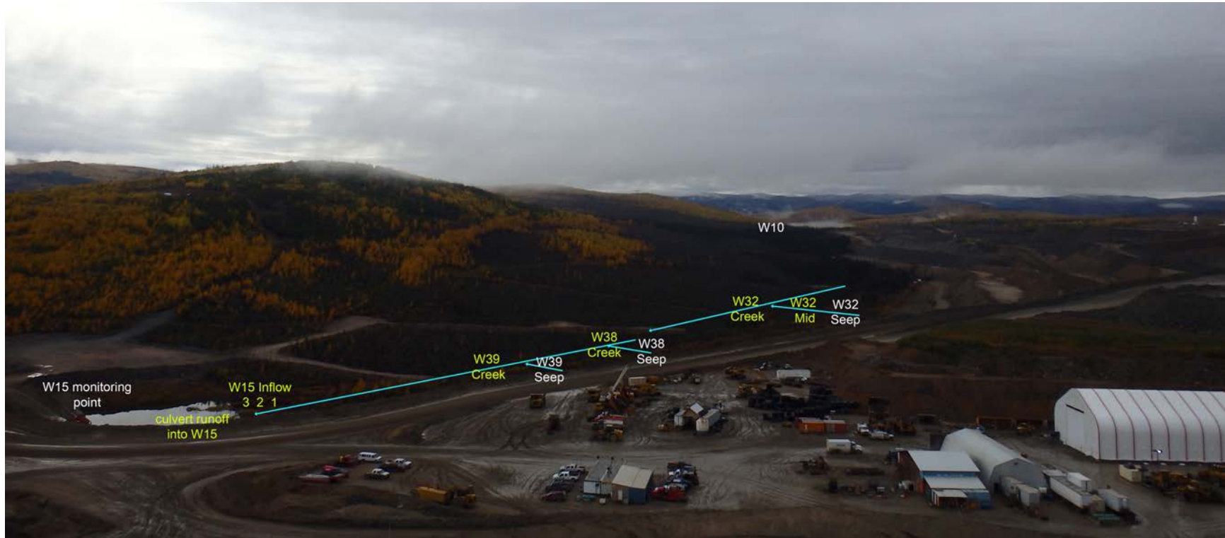
Figure 2: Sampling locations at the Minto mine. All routine monitoring points are indicated in white, while sampling locations unique to this study are shown in yellow. The blue arrows indicate the direction of water flow. The W32 Creek label corresponds to the location of both the W32 Creek and W32 Creek Red.
