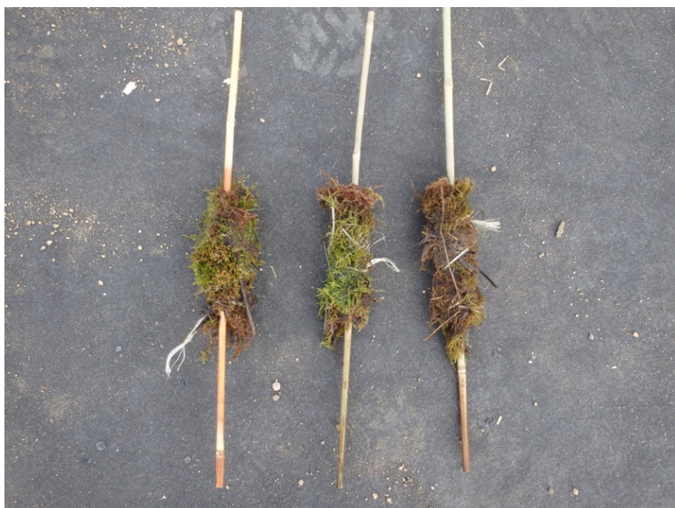
Figure 10. Example of moss tied to stakes, which then were used to make grid in each demonstration-scale CWTS (Figure 4, 11, 12 and Table2).
