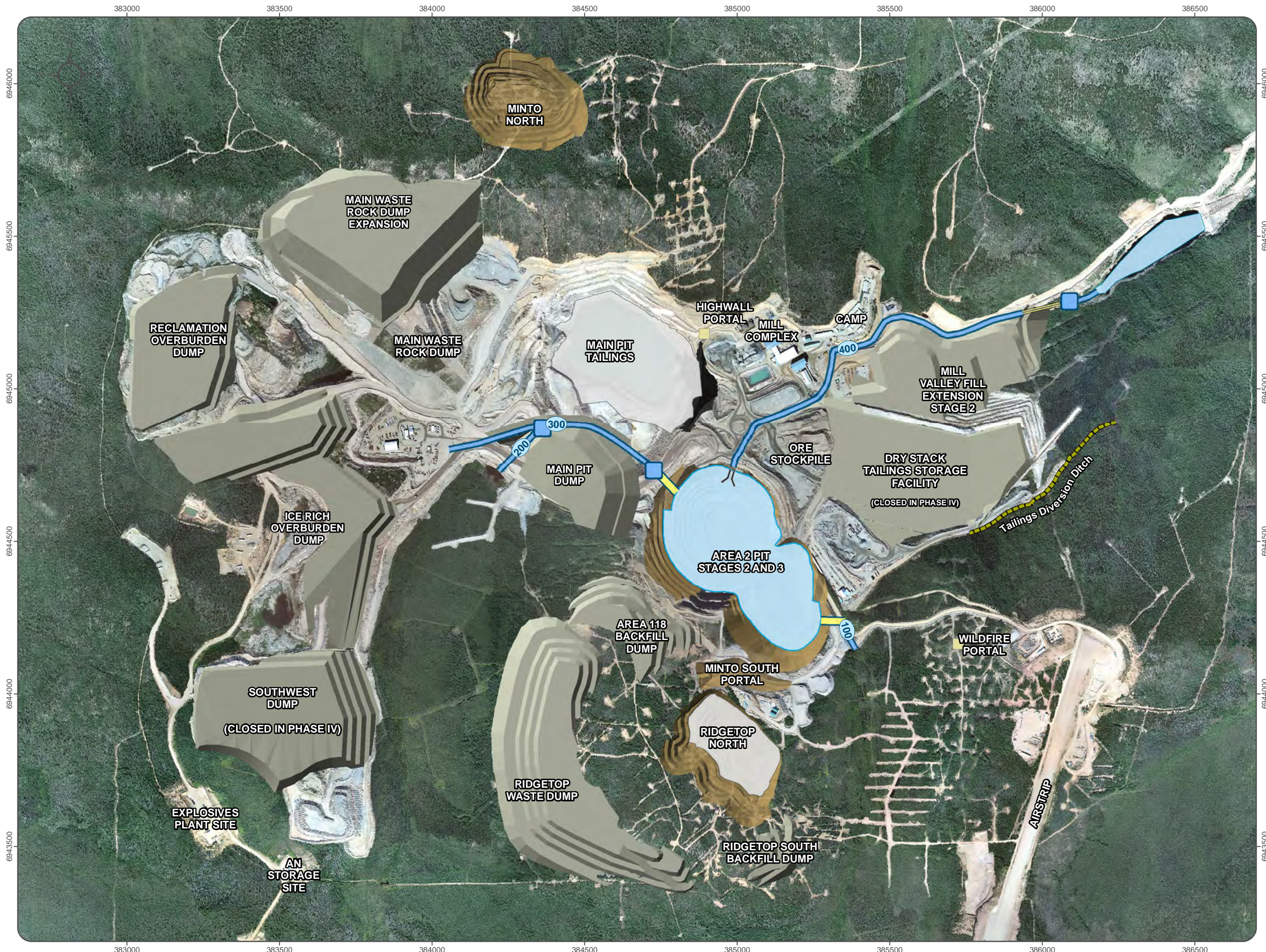
FIGURE 3 - 1 CLOSURE WATER MANAGEMENT LAYOUT
