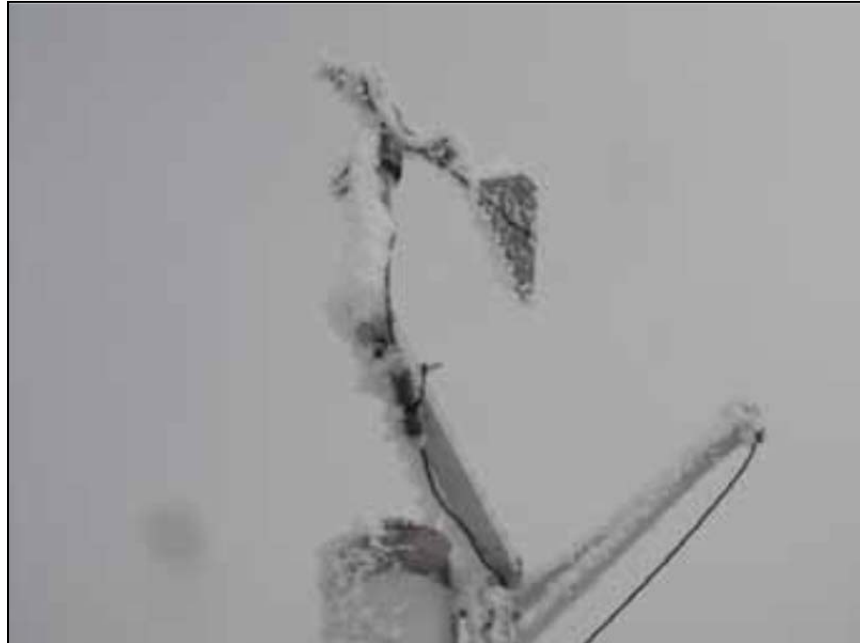
Figure 3-8: Rime Icing Affecting the Minto HOBO Anemometer (Source: EBA 2010).
