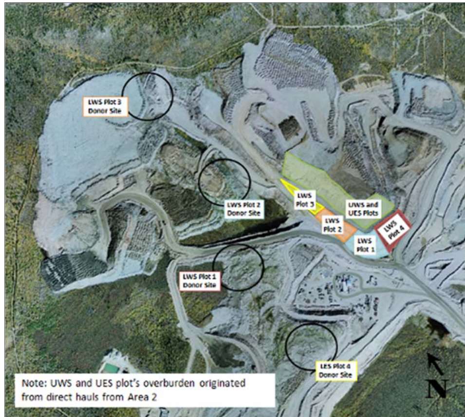
Figure 2-5 Origin of overburden material from ROD placed in distinct plots on the MWD re-contoured rock surface
