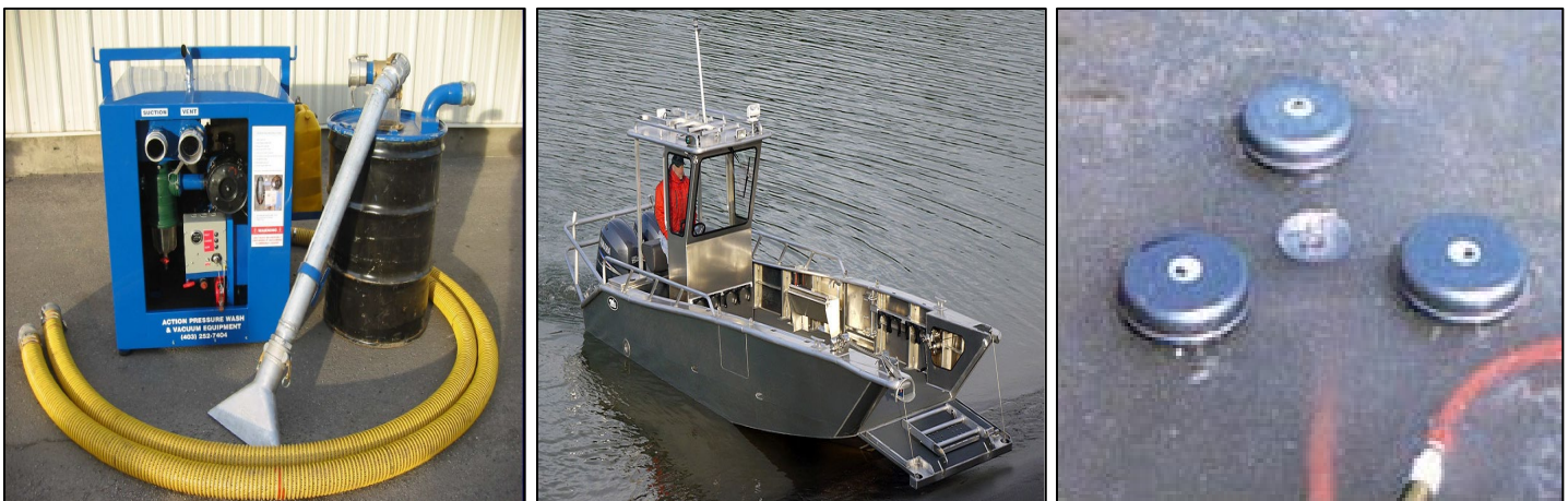
Figure 6-2: In-Viro Drum and vacuum unit, 24' Packman vessel, and Alpha Skimmer for spill response operations.
