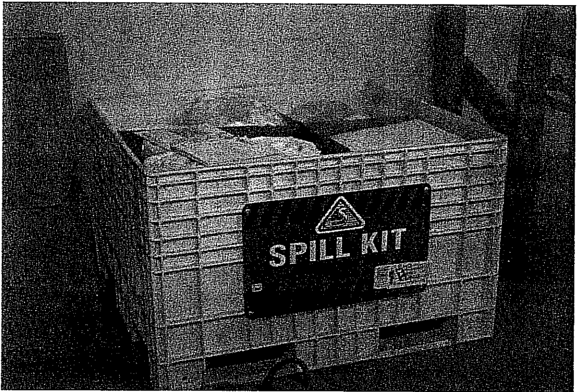
Spill response palletized container filled with adsorbant mats and containment booms. Spare material in adjacent boxes.
