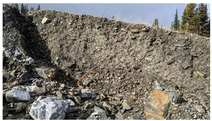
Photo WR-03: Side-wall of the erosion gulley at the base of Jewelbox Waste Dump. The gulley is approximately 2 m deep with vertical sidewalls.
