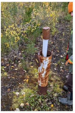
Photo ND-09: Piezometer NDW-4A downstream of the dam toe. The PVC pipe extends above the protective casing. A soup can is used as an end cap and would found displaced during the inspection.
