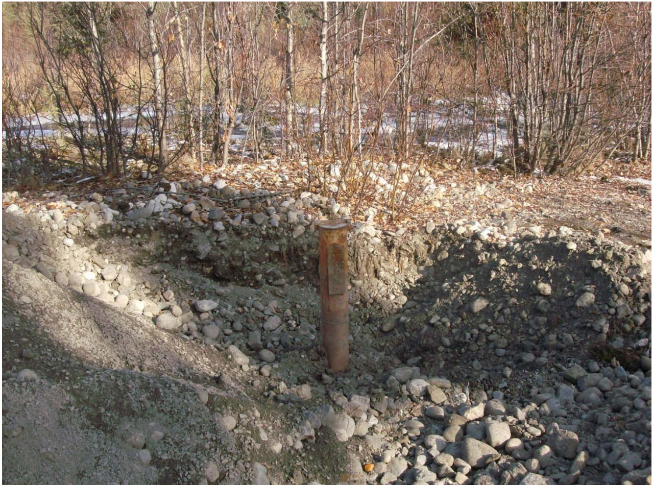
Photo 1: Monitoring Well TH24-91 exposed.
