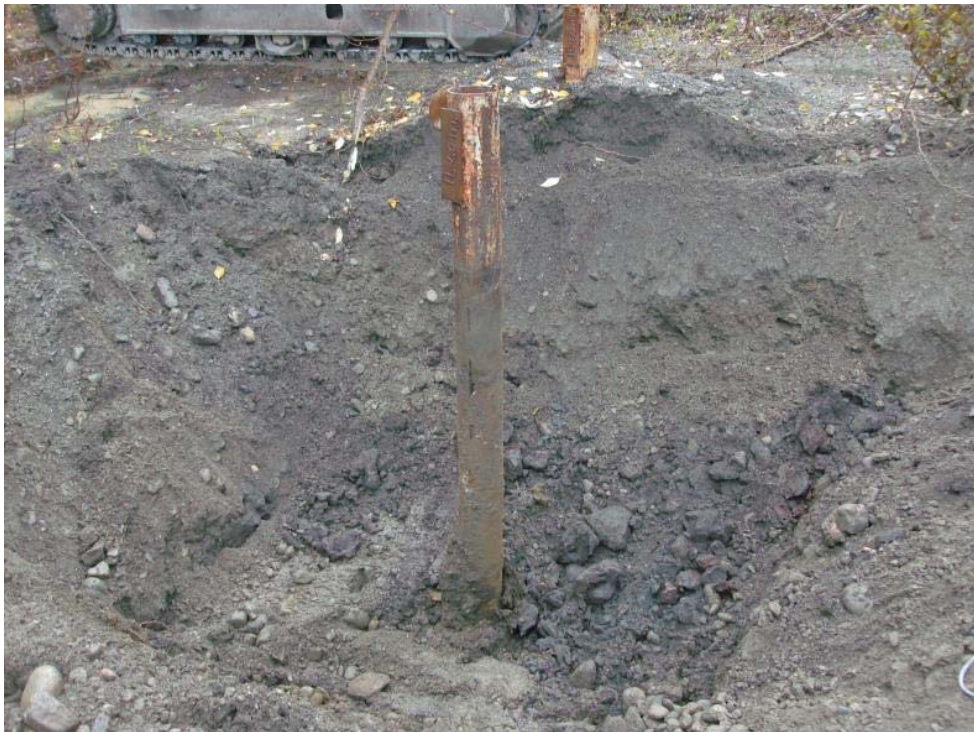
Photo 2: TH07-91 exposed prior to cutting.
