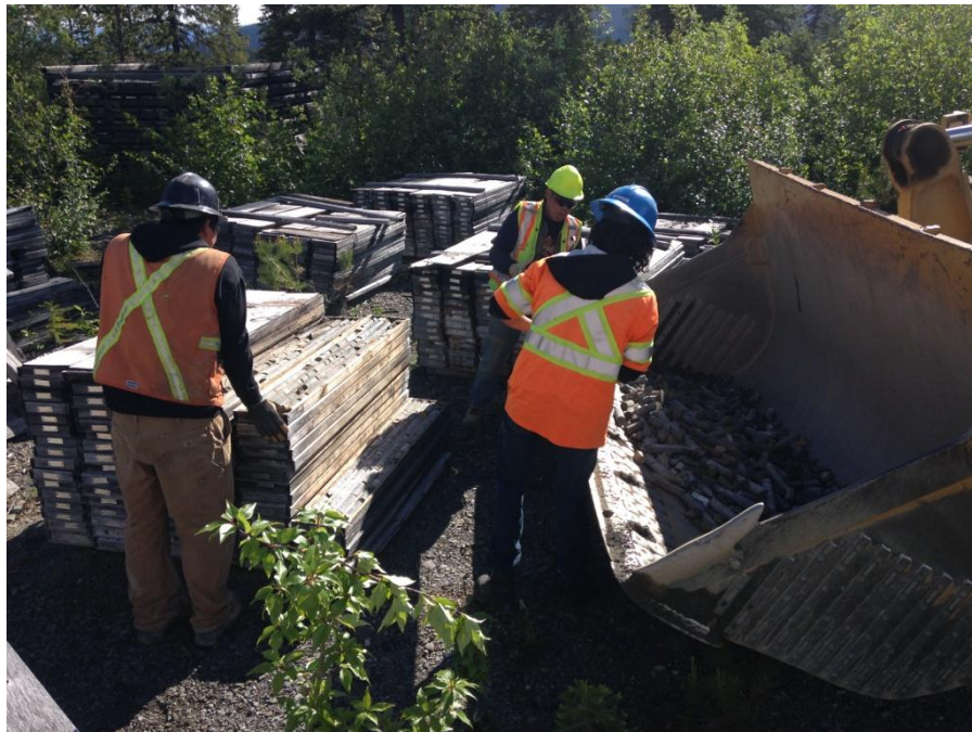
MISC Photograph 8: Labourers extracting core from core racks and placing in loader bucket for haul to Jewelbox for disposal.
