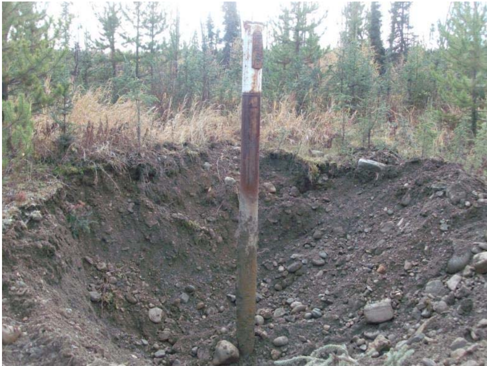
Photo 1: Monitoring Well TH19-91 exposed prior to cutting down.
