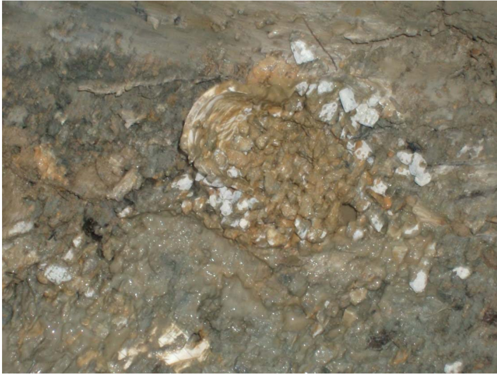
Photo 1: Well GW-1B filled with bentonite after being exposed and cut down.
